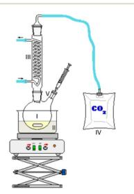
Fig. 2 Closed aging setup for accelerated laboratory aging (setup 2).
