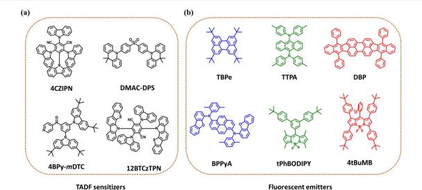
Fig. 3 (a) Molecular structures of TADF emitters used as sensitizers for hyperfluorescent OLEDs. (b) Molecular structures of various blue, green and red fluorescent emitters used as final dopants.
