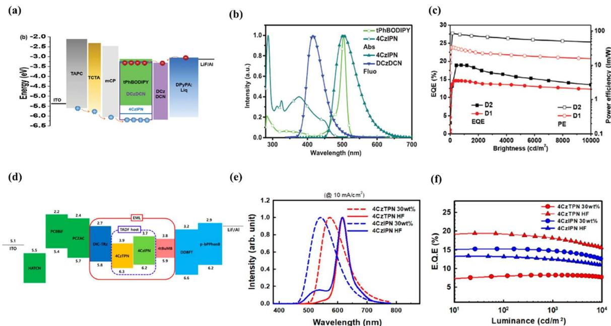
Fig. 5 (a–c) Green hyperfluorescent OLEDs. The device structure used in fabrication, absorption and emission spectra of *t*PhBODIPY and 4CzIPN and the efficiency plot of the devices. Reproduced with permission from ref. 66, John Wiley and Sons, 2020. (d–f) Red hyperfluorescent OLEDs. The device structure of the HF-OLED, electroluminescence spectra of TADF-based and HF-based OLEDs and EQE vs. luminance of the devices. Reproduced with permission from ref. 70, American Chemical Society, 2021.
