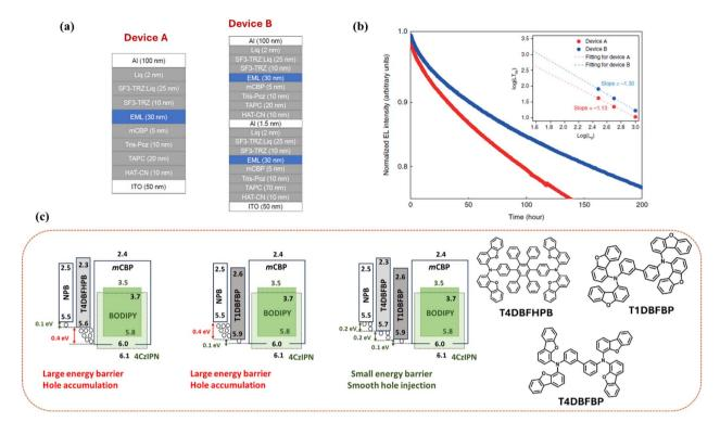
Fig. 11 (a) Device structure of single-unit and two-unit stacked tandem hyperfluorescent OLEDs. (b) Electroluminescence intensity versus operation time at an initial luminance of 1000 cd  $m^{-2}$ . Inset: LT<sub>95</sub> as a function of  $L_0$ . Reproduced with permission from ref. 144, Nature, 2021. (c) Schematic illustration of hole injection behaviour from the HTL to the EML using various HTLs, along with the molecular structures of the respective HTLs used.
