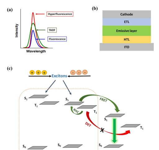
Fig. 2 (a) Spectral behaviour of fluorescent, TADF and hyperfluorescent devices. (b) A simplified device structure of multilayer organic light-emitting diodes: ITO (indium tin oxide)/HTL (hole transporting layer)/emissive layer/ETL (electron transporting layer)/cathode. (c) A schematic diagram of energy transfer processes in a hyperfluorescent device.
