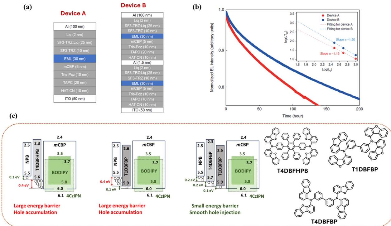
Fig. 11 (a) Device structure of single-unit and two-unit stacked tandem hyperfluorescent OLEDs. (b) Electroluminescence intensity versus operation time at an initial luminance of  $1000 \text{ cd m}^{-2}$ . Inset:  $LT_{95}$  as a function of  $L_0$ . Reproduced with permission from ref. 144, *Nature*, 2021. (c) Schematic illustration of hole injection behaviour from the HTL to the EML using various HTLs, along with the molecular structures of the respective HTLs used.
