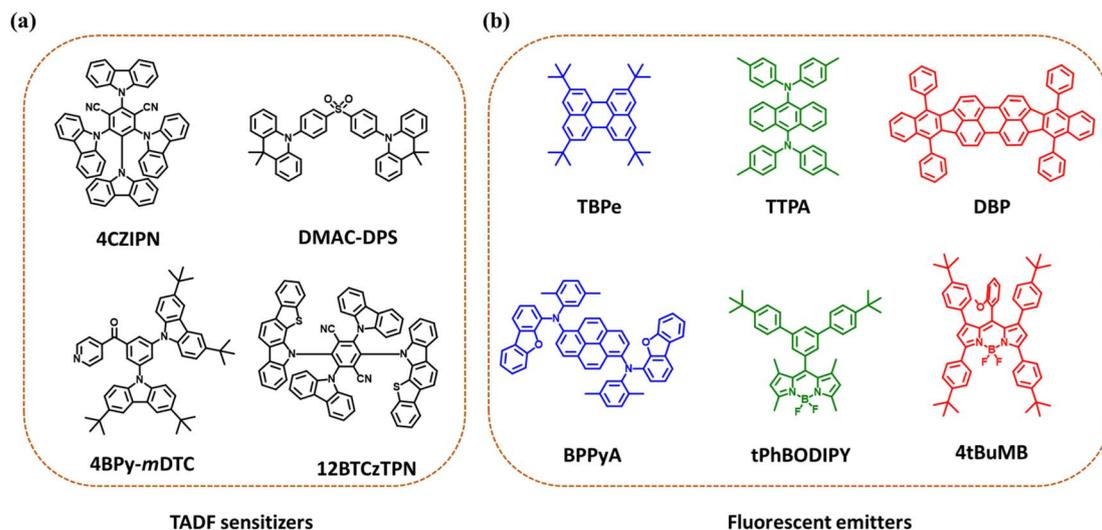
Fig. 3 (a) Molecular structures of TADF emitters used as sensitizers for hyperfluorescent OLEDs. (b) Molecular structures of various blue, green and red fluorescent emitters used as final dopants.
