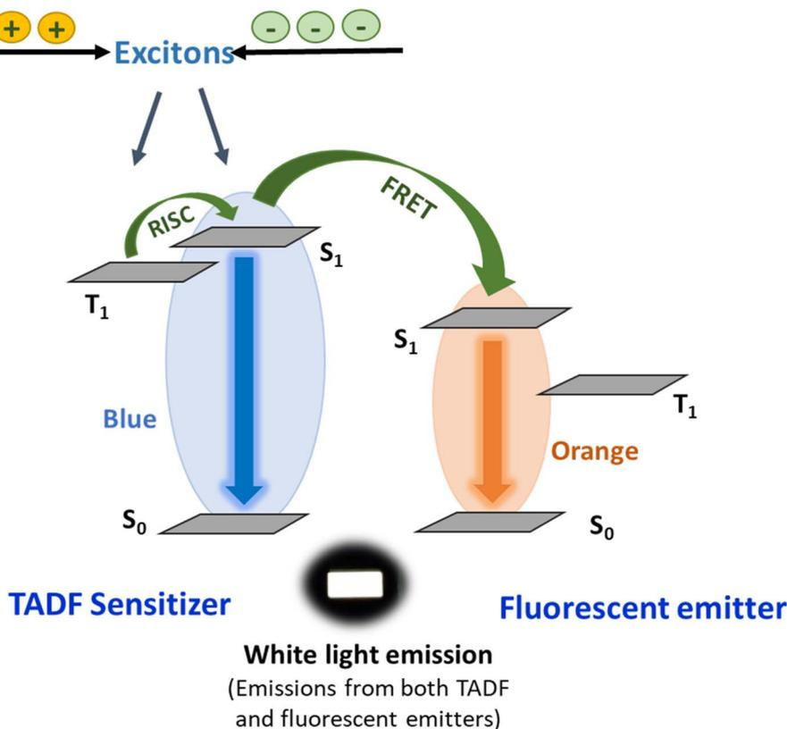
Fig. 6 A schematic representation of white light emission from both the TADF sensitizer and fluorescent emitter.
