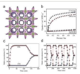
Fig. 42 (a) The structure of UTSA-280. (b) The  $CO_2/CH_4$  sorption isotherms of UTSA-280 at 273 and 298 K. (c) and (d) The breakthrough curves and cycles of UTSA-280 for  $CO_2/CH_4$  (1:1). Reproduced from ref. 245 with permission from Wiley, Copyright 2020.
