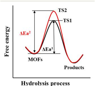
Scheme 3 The definition and optimization of the kinetic stability of MOFs to water. Black line represents the kinetic stability of a given MOF to water, which refers to the  $\Delta Ea^1$  (activation energy) of its hydrolysis reaction. The red line represents the optimized kinetic stability of the MOF through enhancing its activation energy ( $\Delta Ea^2 > \Delta Ea^1$ ).
