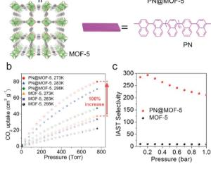
Fig. 36 (a) Introducing hydrophobic polynaphthylene (PN) into MOF-5 through the polymerization of DEB. (b) The CO<sub>2</sub> adsorption isotherms of MOF-5 and PN@MOF-5 at different temperatures. (c) The IAST selectivity of MOF-5 and PN@MOF-5 for a CO<sub>2</sub>/N<sub>2</sub> mixture (14: 86) at 273 K. Reproduced from ref. 222 with permission from the American Chemical Society, Copyright 2016.
