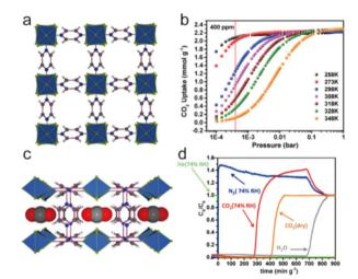
Fig. 38 (a) The structure of NbOFFIVE-1-Ni. (b) The  $\rm CO_2$  sorption isotherms of NbOFFIVE-1-Ni at different temperatures. (c) The  $\rm CO_2$  adsorption sites in NbOFFIVE-1-Ni. (d) The breakthrough curves with the mixed-gas  $\rm CO_2/N_2$  (1/99) at 1 bar and 298 K in both dry and humid environments. Reproduced from ref. 191 with permission from the American Chemical Society, Copyright 2016.
