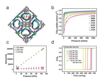
Fig. 39 (a) The structure of FJI-H38. (b) The  $CO_2$  sorption isotherms of FJI-H38 at different temperatures. (c) The IAST selectivity of FJI-H38 for  $CO_2/N_2$  at various partial pressures. (d) The breakthrough curves of FJI-H38 for  $CO_2/N_2$  (1:99) under different humid conditions. Reproduced from ref. 190 with permission from Wiley, Copyright 2023.
