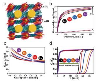
Fig. 32 (a) The structure of NKMOF-3-Ln. (b)–(d) The  $\rm CO_2/N_2$  adsorption isotherms,  $\rm CO_2$  adsorption enthalpy, and breakthrough curves of  $\rm CO_2/N_2$  (15/85) mixtures at 298 K. Reproduced from ref. 212 with permission from the American Chemical Society, Copyright 2019.
