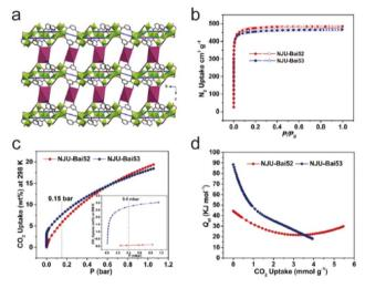
Fig. 37 (a) The structure of NJU-Bai52 and NJU-Bai53. (b) The  $\rm N_2$  sorption isotherms of NJU-Bai53 (77 K) before and after water treatment. (c) The  $\rm CO_2$  adsorption isotherms of NJU-Bai52 and NJU-Bai53 at 298 K. (d) The adsorption enthalpy of NJU-Bai52 and NJU-Bai53 for  $\rm CO_2$ . Reproduced from ref. 233 with permission from the American Chemical Society, Copyright 2019.
