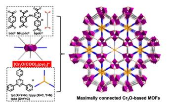
Fig. 13 The structural components, together with the framework viewed along the c axis.  $NH_2bdc^{2-}=2$ -aminoterephthalate, bpdc $^{2-}=$  biphenyl-4,4'-dicarboxylate), tpt = 2,4,6-tri(4-pyridyl)-1,3,5-triazine, tpbz = 1,3,5-tri(4-pyridyl)-benzene, and tppy = 2,4,6-tris(4-pyridyl) pyridine. Reproduced from ref. 153 with permission from the American Chemical Society, Copyright 2021.
