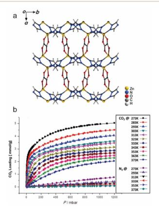
Fig. 35 (a) The structure of CALF-20. (b) The  $\rm CO_2$  and  $\rm N_2$  isotherms of CALF-20 at different temperatures. Reproduced from ref. 217 with permission from the Advancement of Science, Copyright 2021.
