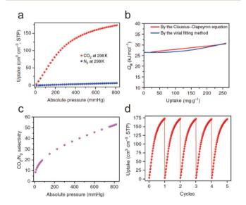
Fig. 34 (a) The  $\rm CO_2$  and  $\rm N_2$  adsorption isotherms for FJI-H14 at 298 K. (b) The isosteric heat of  $\rm CO_2$  adsorption ( $\rm Q_{st}$ ) for FJI-H14. (c) The IAST selectivity of FJI-H14 for  $\rm CO_2/N_2$  (15:85). (d) 5 Cycles of  $\rm CO_2$  adsorption for FJI-H14 at 298 K. Reproduced from ref. 136 with permission from Springer Nature, Copyright 2017.
