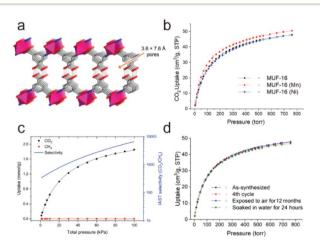
Fig. 44 (a) The structure of MUF-16. (b) The CO<sub>2</sub> adsorption isotherms of MUF-16s at 293 K. (c) The IAST selectivity of MUF-16 for CO<sub>2</sub>/CH<sub>4</sub> (50:50) at 293 K. (d) The CO<sub>2</sub> adsorption isotherms of MUF-16 at 293 K, after 4 consecutive sorption cycles, 12 months of exposure to air with 80% RH, and 24 hours of immersion in water. Reproduced from ref. 265 with permission from Springer Nature, Copyright 2021.
