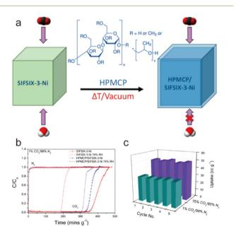
Fig. 41 (a) Coating HPMCP on SIFSIX-3-Ni. (b) The breakthrough curves of SIFSIX-3-Ni and HPMCP/SIFSIX-3 for  $CO_2/N_2$  (1:99) under different humid conditions. (c) The HPMCP/SIFSIX-3-Ni recyclability tests for humid 1%  $CO_2/99\%$   $N_2$  and 15%  $CO_2/85\%$   $N_2$  gas mixtures (regeneration at 80 °C). Reproduced from ref. 254 with permission from the American Chemical Society, Copyright 2020.
