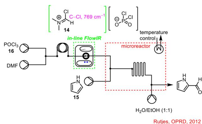
**Scheme 5** In-line FlowIR flow cell used to monitor conversion of  $\text{POCl}_3$  **16** in the telescoped process to synthesise 2-formylpyrrole **17** (ref. 43).
