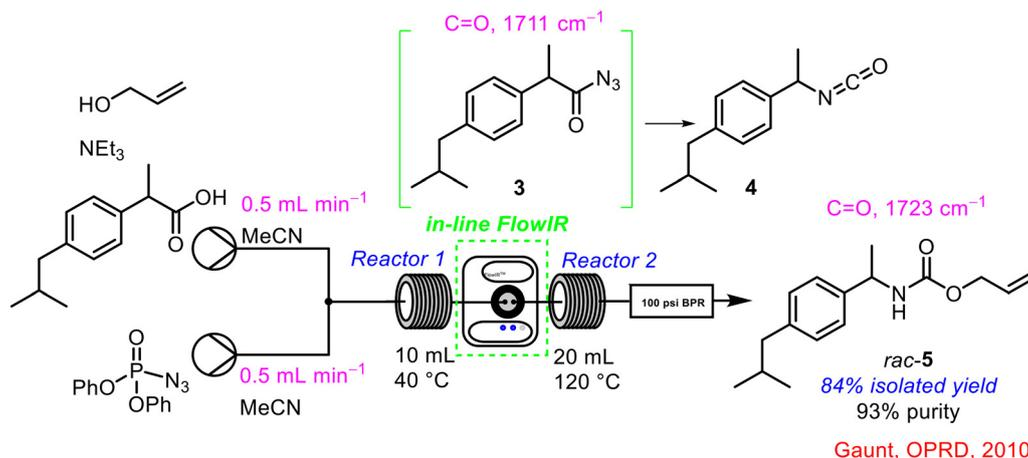
Scheme 2 In-line FTIR analysis of carbamate 5 synthesis reported by Gaunt and co-workers.<sup>35</sup>
