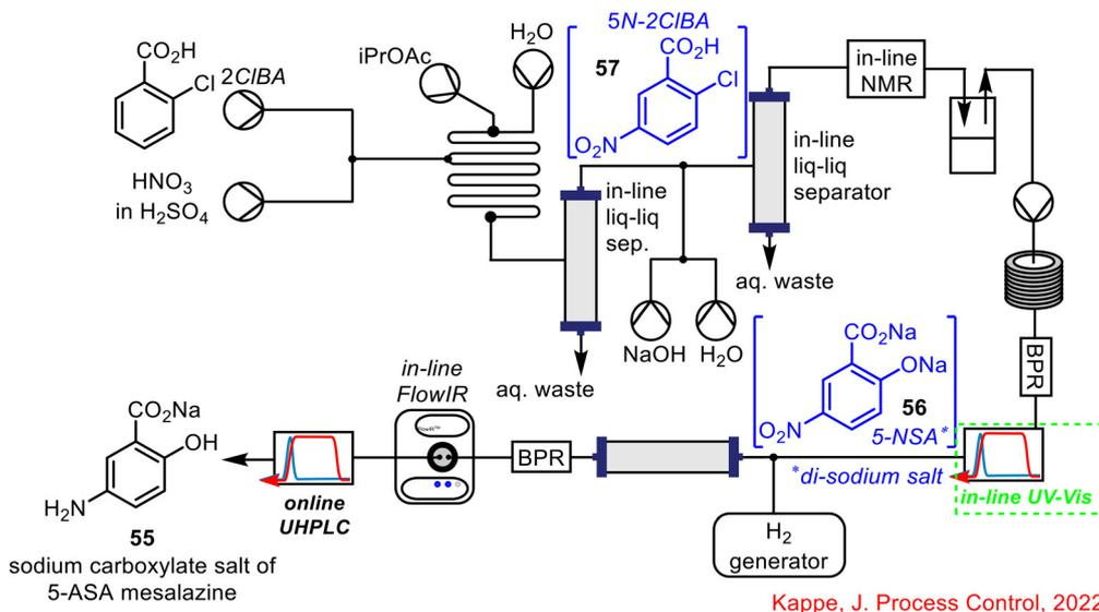
**Scheme 21** Telescoped synthesis of sodium carboxylate salt of mesalazine reported by Kappe.<sup>16,17,55</sup>
