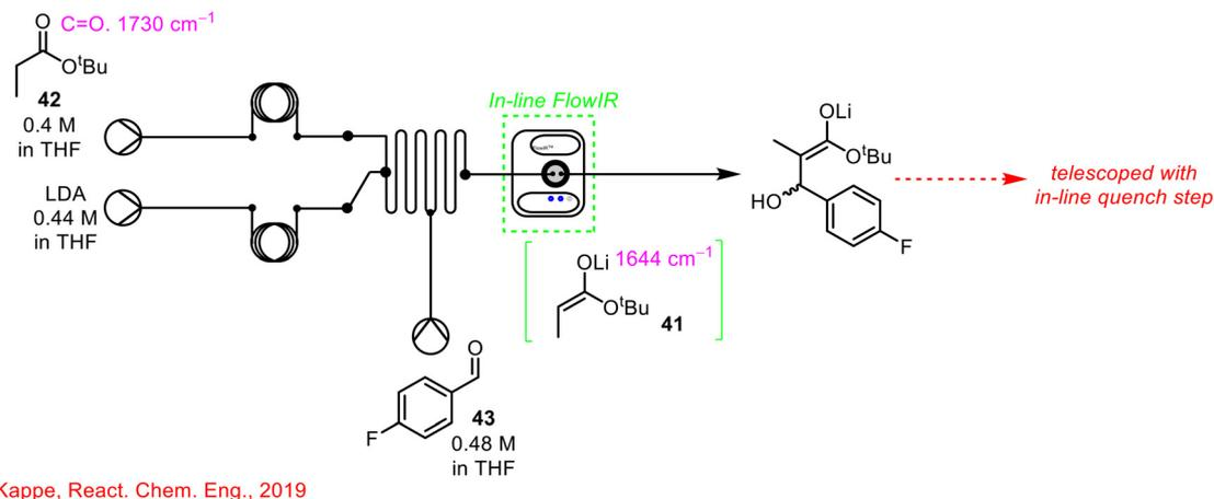
**Scheme 15** Simplified schematic of in-line FlowIR cell used by Kappe and co-workers for organolithium transformation.<sup>11</sup>
