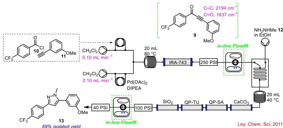
**Scheme 4** FlowIR to enhance production and safety of telescoped process by Ley and co-workers.<sup>37</sup>
