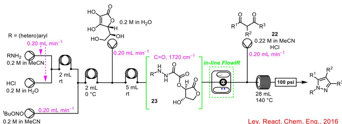
**Scheme 9** In-line FlowIR used to develop the four-step telescoped continuous synthesis of pyrazoles.<sup>48</sup>
