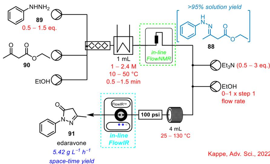
**Scheme 35** Telescoped two-step synthesis of API edaravone using in-line FlowNMR to monitor initial imine formation step.<sup>76</sup>
