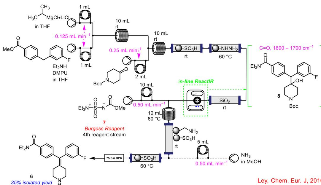
Scheme 3 Use of in-line FlowIR flow cell in the synthesis of a  $\delta$ -opioid receptor agonist 6 by Ley and co-workers.<sup>36</sup>
