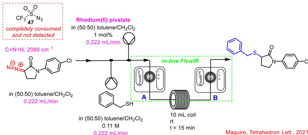
**Scheme 17** Incorporation of an in-line FlowIR cell post-diazo transfer reaction and post-S-H insertion reaction by Maguire and co-workers.<sup>57</sup>
