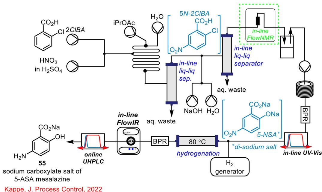
**Scheme 34** Telescoped synthesis of the sodium carboxylate salt of mesalazine **55** reported by Kappe utilising in-line FlowNMR, in-line UV-vis, in-line FlowIR and online UHPLC as process monitoring tools.<sup>16,17,55</sup>
