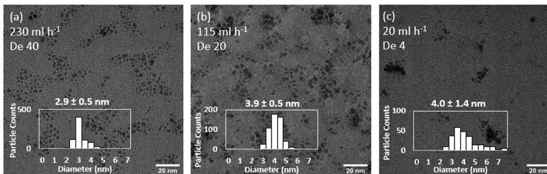
Fig. 4 Effect of total flowrate of (a) 230 ml h<sup>-1</sup>, (b) 115 ml h<sup>-1</sup> and (c) 20 ml h<sup>-1</sup> on the size and distribution of continuously synthesised Ru NPs. Representative TEM images. Experiments 1–3, Table 3.
