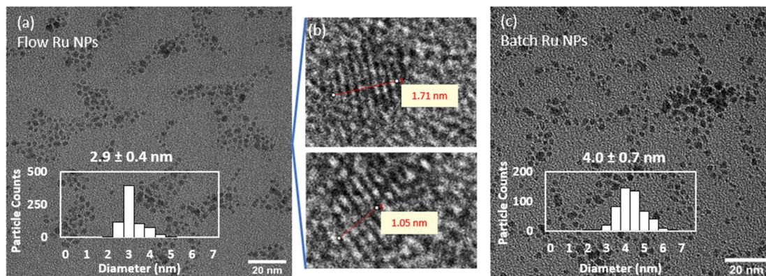
Fig. 2 Representative TEM images of (a) flow synthesis of Ru NPs collected in  $\text{HNO}_3$  (b) lattice fringes from flow-synthesised Ru NPs showing spacing of 0.21 nm corresponding to hexagonal close-packed Ru(0), and (c) comparative batch synthesis. Conditions: 1.25 mM  $\text{Ru}(\text{NO})(\text{NO}_3)_3$  and 3.13 mM  $\text{NaBH}_4$ , pH upon mixing: 9.5, pH after  $\text{HNO}_3$  quench: 1.3, 25 °C.
