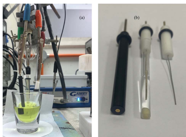
Fig. 2 Image shows photograph of (a) gold disk working electrode, Ag/AgCl reference electrode and platinum wire electrode in a conventional experimental setup with larger volume 10 mL of potassium ferricyanide solution in a glass vial. Figure (b) meanwhile shows the cross-sectional image of the gold disk working electrode, Ag/AgCl reference electrode and the platinum wire counter electrodes.
