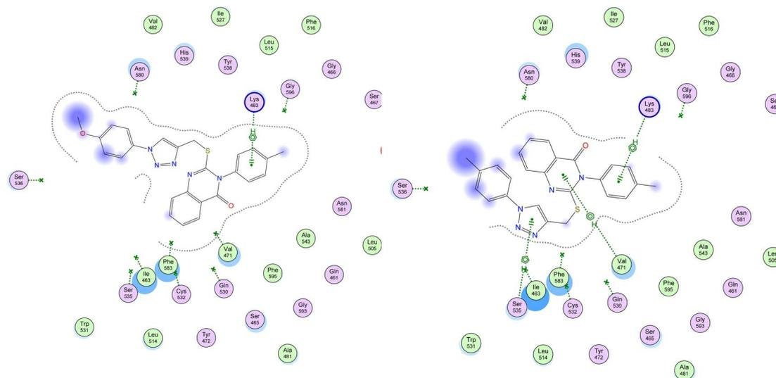
Fig. 9 Depicted 2D figures of binding interactions of compounds **8g** and **8h** within active site of BRAF<sup>V600E</sup> (PDB ID: 4RZV) showing pi-H bonds as green-dotted lines with LYS 483, VAL 471, and SER 535.
