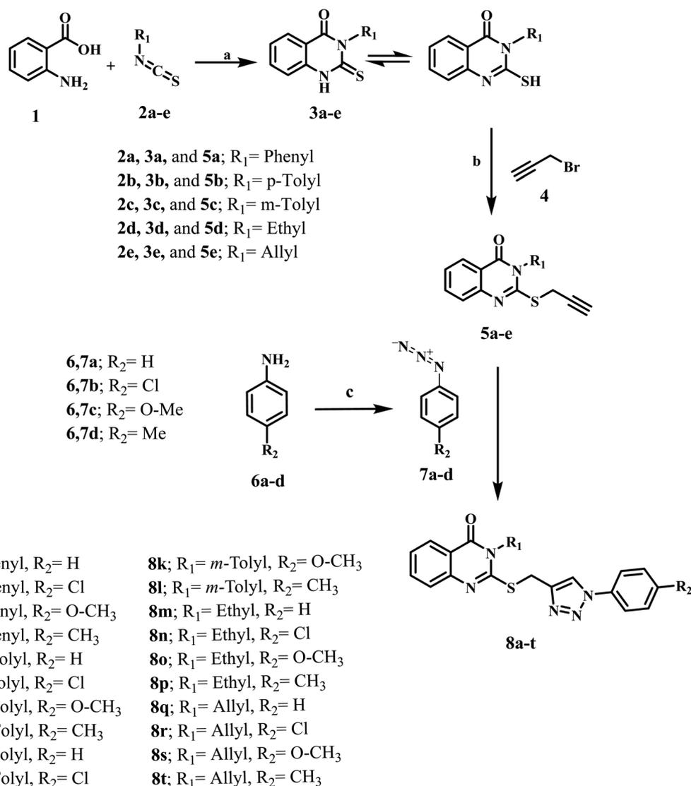
**Scheme 1** Synthesis of the new target compounds **8a–t**. Reagents and conditions: (a) TEA, ethanol, reflux (8–12 h), (b) K<sub>2</sub>CO<sub>3</sub>, DMF, stirring (24 h), (c) 1-NaNO<sub>2</sub>, HCl, 2-NaN<sub>3</sub> (d) sodium ascorbate, CuSO<sub>4</sub>·5H<sub>2</sub>O, THF, reflux (24–48 h).
