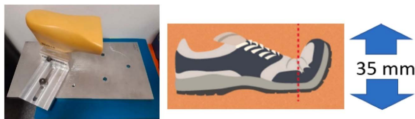
Fig. 11 The setup used for the stiffness test. A stiffness test was performed using the Instron 3360 universal testing machine. Footwear was tested with no insole. Distance of extension – 35 mm. 161 Copyright 2022, Elsevier.
