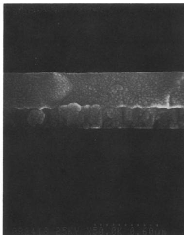
Fig. 4 Cross-section of Ta<sub>2</sub>O<sub>5</sub> thin film prepared by the sol-gel method using photo-irradiation (Reproduced from ref. 44 with permission from Elsevier copyright [2024]).
