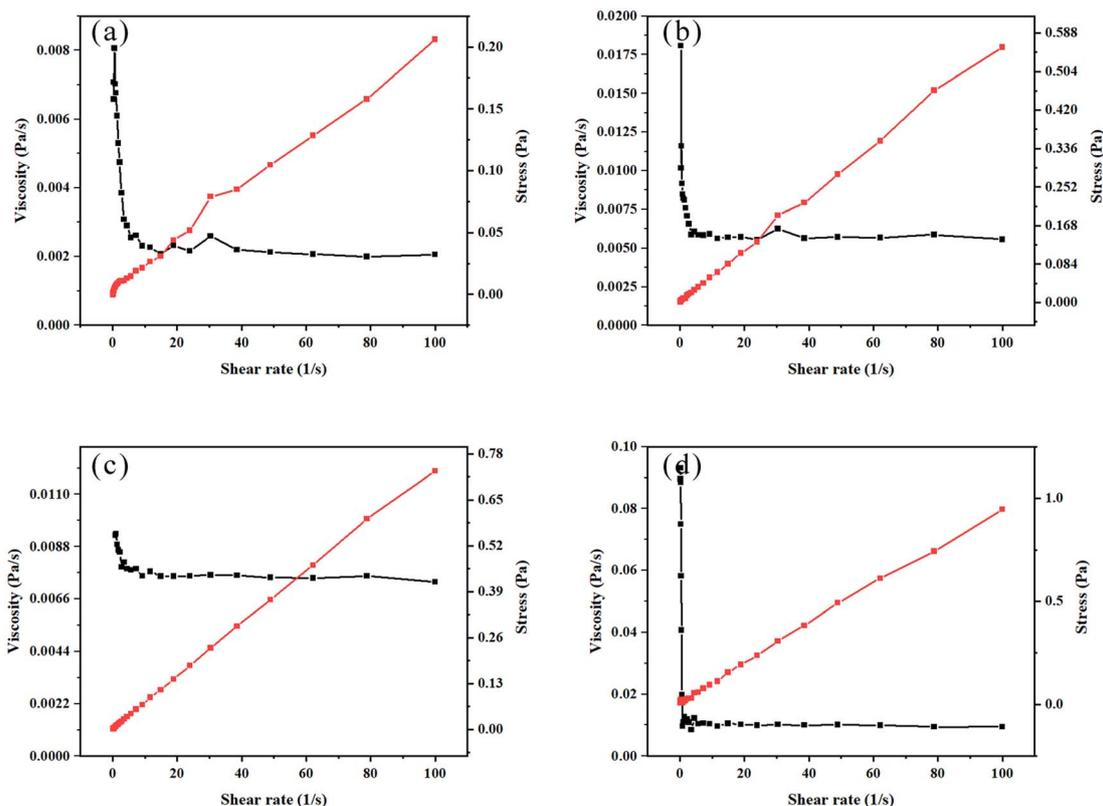
Fig. 13 The relationship between ink viscosity, shear stress, and shear rate as a function of sodium alginate content in the additive (a)  $20 \text{ wt\%}$  sodium alginate content ratio (b)  $30 \text{ wt\%}$  sodium alginate content ratio (c)  $40 \text{ wt\%}$  sodium alginate content ratio (d)  $50 \text{ wt\%}$  sodium alginate content ratio.
