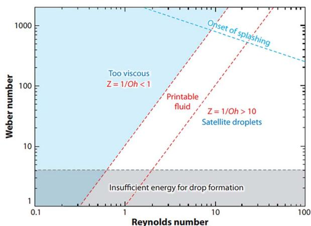
Fig. 16 The allows stable printing range.<sup>41</sup>
