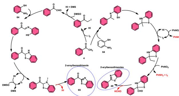
Scheme 38 Mechanism for the synthesis of aroylbenthioazole **65** and arylbenthiozoles **66** using  $I_2$ -DMSO system.
