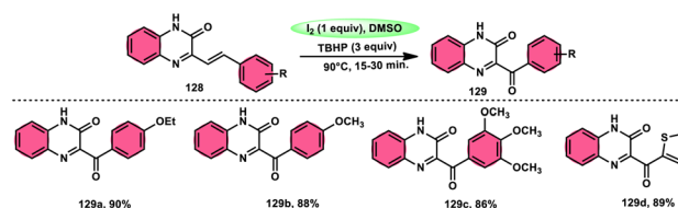
Scheme 78 I 2 /DMSO-mediated metal-free reaction.
