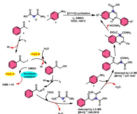
Scheme 9 Mechanism of 2-arylquinoline-4-carboxylate 13.
