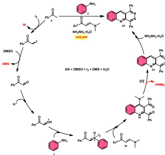
Scheme 20 Mechanism for the synthesis of quinolines **34** and **35**.
