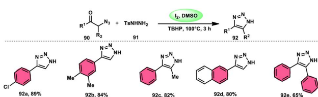
Scheme 52 Synthesis of triazoles 92 and selected examples.
