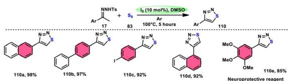
Scheme 67 Synthesis of thiadiazoles **110** using  $I_2$ /DMSO system.
