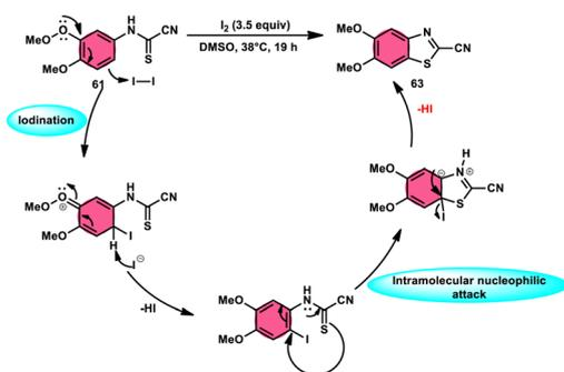
Scheme 36 Synthesis and mechanism of 2-cyanobenzothiazoles **63**.
