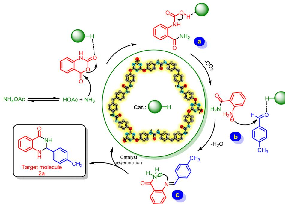
Scheme 4 A plausible mechanism for the preparation of 2f in the presence of urea-rich POP as catalyst.
