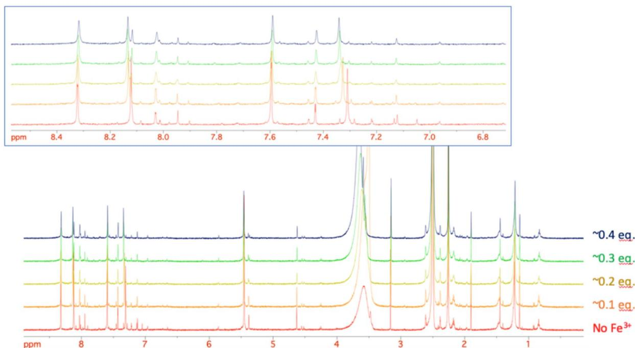
Fig. 3 The stacking plot of NMR spectra of **18b** after stepwise addition of FeCl<sub>3</sub> to a DMSO solution of **18b**. The inset shows the aromatic region of **18b**.
