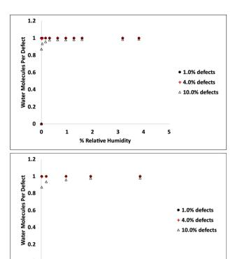
Fig. 2 Amount of water adsorbed per defect (S vacancy) at 298 K and low humidity levels.
