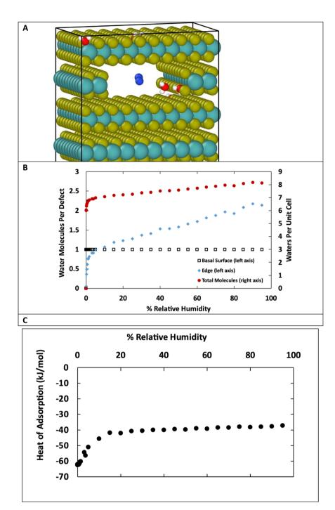
Fig. 11 (A) Snapshot from GCMC simulation in  $MoS_2$  with 1% defects, including edge and surface defects. Colors: yellow S, teal Mo, red O, white H, blue N. (B) Adsorption isotherm for water at 298 K on  $MoS_2$  structure containing both basal surface and edge defects. This structure has 6 surface defects and 1 edge defect, for 7 total defects, representing 1% of the total S atoms. (C) Heat of adsorption of water in kJ mol<sup>-1</sup>.
