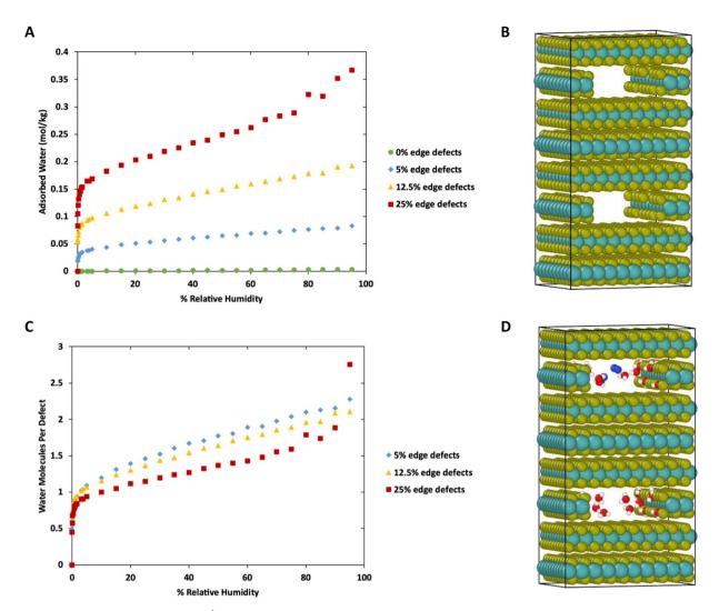
Fig. 8 (A) Adsorption isotherms in mol  $kg^{-1}$  for water in MoS<sub>2</sub> with edge defects. Temperature is 298 K. (B) Visualization of MoS<sub>2</sub> structure with edge defects. (C) Adsorption isotherms in water per defect site at 298 K. (D) Visualization of water adsorbed onto MoS<sub>2</sub> at 298 K and 90% RH. Colors: yellow S, teal Mo, red O, white H, blue N. System size:  $31.475 \times 31.475 \times 48.288$  Å.
