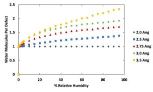
**Fig. 6** Adsorption isotherms for water at 298 K in MoS<sub>2</sub> with lamellae separation increased from the ideal distance by 2.0, 2.5, 2.75, 3.0, and 3.5 Å. (A) shows the isotherms normalized as water per Mo atom for defect-free MoS<sub>2</sub> compared to MoS<sub>2</sub> with 1% defects (B) shows the isotherms normalized as water per defect for MoS<sub>2</sub> with 1% random S vacancy defects.
