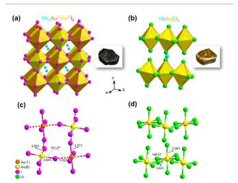
**Fig. 1** Single-crystal X-ray diffraction analysis of (a)  $Rb_2Au_2l_6$  and (b)  $RbAuCl_4$ . The blue, orange, gold, red, purple, and green spheres represent Rb,  $Au^I$ ,  $Au^{III}$ , I, and Cl atoms, respectively. The insets show the photographs of the crystals. (c and d) Bond lengths and angles of  $Rb_2Au_2l_6$  and  $RbAuCl_4$ . Rb atoms are omitted in the schematic diagram for the ease of structural description.
