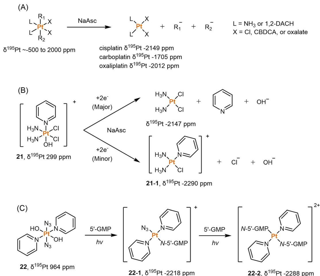
**Scheme 2** Monitoring the Pt(II) complexes generated as reduction products by  $^{195}\text{Pt}$  NMR. (A) Reduction pathway of typical Pt(IV) complexes (where CBDCA = 1,1-cyclobutanedicarboxylate; 1,2-DACH = 1,2-diaminocyclohexane). (B) Reduction pathway of pyridinyl-Pt(IV) complex **21**. (C) Reduction pathway of azido-Pt(IV) complex **22**.
