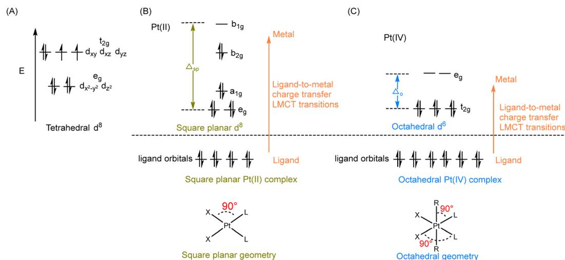
Fig. 3 (A) The d-orbital splitting diagrams for tetrahedral  $d^8$  complexes. (B) The d-orbital splitting diagrams and the ligand-to-metal charge transfer (LMCT) (upper), as well as the geometry (lower) of square planar  $d^8$  Pt(II) drugs. (C) The d-orbital splitting diagrams and the ligand-to-metal charge transfer (LMCT) (upper), as well as the geometry (lower) of octahedral  $d^6$  Pt(IV) prodrugs.
