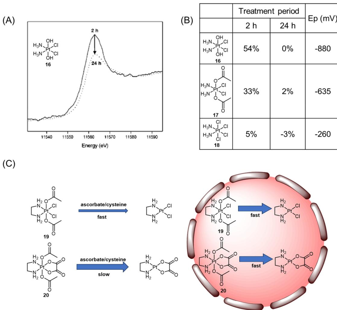
**Fig. 10** (A) Normalized XANES spectra of A2780 cells incubated with Pt(IV) complex **16** after 2 h (solid line) and 24 h (dotted line). Adapted with permission from ref. 71. Copyright 2003, American Chemical Society. (B) Proportion of Pt(IV) ( $\pm 5\%$ ) remaining after incubation of complexes with A2780 cells and their reduction potentials ( $E_p$ ). (C) The reduction of complexes **19** and **20** in various biological contexts.
