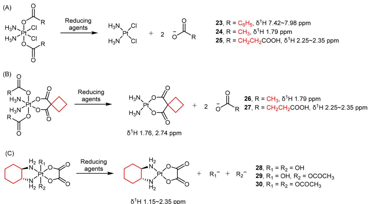
**Scheme 3** Monitoring the reduction of cisplatin-, carboplatin- and oxaliplatin-based Pt(IV) complexes by  $^1\text{H}$  NMR. Respectively, (A) the hydrogen on axial ligands, (B) both axial ligands and CBDCA, and (C) 1,2-DACH were detected.
