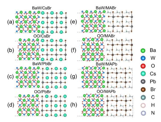
Fig. 1 Schematic illustration of the perovskite/BaWO<sub>4</sub> interfaces: (a) BaW/CsBr, (b) OO/CsBr, (c) BaW/PbBr, (d) OO/PbBr, (e) BaW/MABr, (f) OO/ CsBr, (g) BaW/MAPb, and (h) OO/MAPb.
