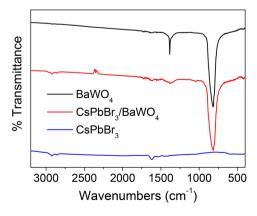
Fig. 8 FT-IR patterns of CsPbBr<sub>3</sub>, BaWO<sub>4</sub>, and CsPbBr<sub>3</sub>/BaWO<sub>4</sub>.
