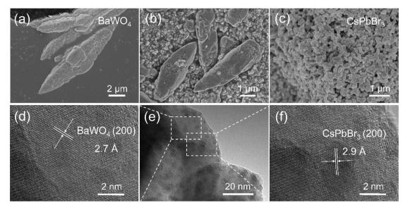
Fig. 9 SEM images of (a) BaWO<sub>4</sub>, (b) CsPbBr<sub>3</sub>/BaWO<sub>4</sub>, and (c) CsPbBr<sub>3</sub>; TEM images of (d) BaWO<sub>4</sub>, (e) CsPbBr<sub>3</sub>/BaWO<sub>4</sub>, and (f) CsPbBr<sub>3</sub>.
