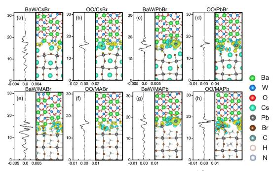
Fig. 3 Plane-averaged electron density difference  $\Delta \rho(z)$  and 3D charge density difference (0.002 e Å<sup>-3</sup>) of the relaxed perovskite/BaWO<sub>4</sub> interfaces: (a) BaW/CsBr, (b) OO/CsBr, (c) BaW/PbBr, (d) OO/PbBr, (e) BaW/MABr, (f) OO/CsBr, (g) BaW/MAPb, and (h) OO/MAPb.
