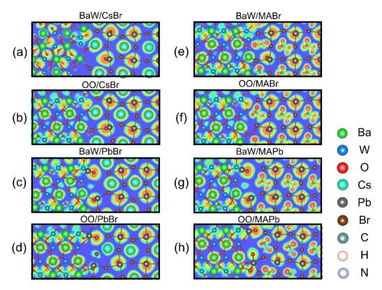
Fig. 2 ELF of the relaxed perovskite/BaWO<sub>4</sub> interfaces: (a) BaW/CsBr, (b) OO/CsBr, (c) BaW/PbBr, (d) OO/PbBr, (e) BaW/MABr, (f) OO/CsBr, (g) BaW/MAPb, and (h) OO/MAPb.
