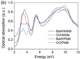
Fig. 6 Absorption coefficients of the relaxed perovskite/BaWO<sub>4</sub> interfaces: (a) CsPbBr<sub>3</sub>/BaWO<sub>4</sub> and (b) MAPbBr<sub>3</sub>/BaWO<sub>4</sub>.
