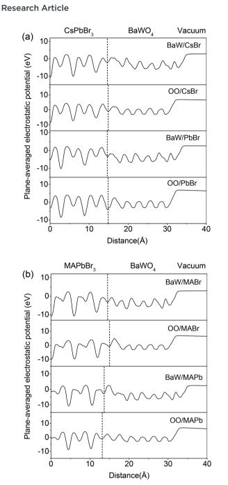
Fig. 4 Plane-averaged electrostatic potential of the relaxed perovskite/ BaWO<sub>4</sub> interfaces: (a) CsPbBr<sub>3</sub>/BaWO<sub>4</sub> and (b) MAPbBr<sub>3</sub>/BaWO<sub>4</sub>.
