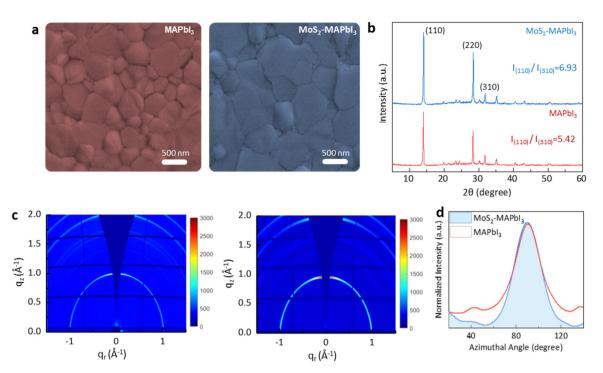
Fig. 3 Crystallization of MoS<sub>2</sub>-MAPbI<sub>3</sub>. (a) SEM images of the MAPbI<sub>3</sub> and MoS<sub>2</sub>-MAPbI<sub>3</sub> films. (b) XRD patterns of the MAPbI<sub>3</sub> film and MoS<sub>2</sub>-MAPbI<sub>3</sub> film. (c) 2D GIWAXS patterns for the MAPbI<sub>3</sub> and MoS<sub>2</sub>-MAPbI<sub>3</sub> films. (d) Azimuthal pole plot of (110) diffraction for the MoS<sub>2</sub>-MAPbI<sub>3</sub> and MAPbI<sub>3</sub> films prepared under the same conditions.
