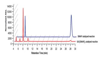
**Fig. 1** HPLC chromatograms for the acetylation of glucopyranoside **40**. Chromatography conditions: Shimadzu Shim-pack (UC-X-Sil) 5  $\mu$ m column, EtOAc-hexane = 60:40, flow rate 1 mL min<sup>-1</sup>, PDA detector (254 nm), retention times: 7.6 min (major isomer **41**), 27.7 min (starting material **40**) and the remaining peaks correspond to the minor isomers.
