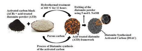
Fig. 1 Diagram illustrating the formation of diatomite synthesized activated carbon (DSAC). This figure has been adapted/reproduced from ref. 42 with permission from Elsevier, copyright 2018.
