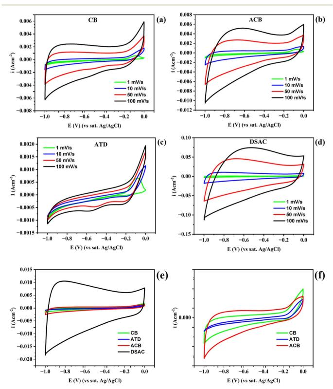
Fig. 7 Cyclic voltammetry curves for (a) CB, (b) ATD, (c) ACB, and (d) DSAC at scan rates of 1, 10, 50, and 100 mV s $^{-1}$  within a voltage range of -1to 0. (e) Overlaid plots for all the electrode materials at a scan rate of  $1 \text{ mV s}^{-1}$  within a voltage range of -1 to 0 and (f) expanded version of the combined plot labelled (e) without DSAC.
