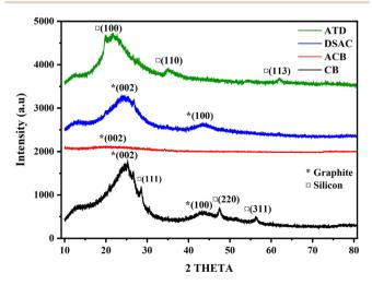
Fig. 3  $\,$  X-ray diffraction analysis of the CB, ACB, ATD, and DSAC samples.
