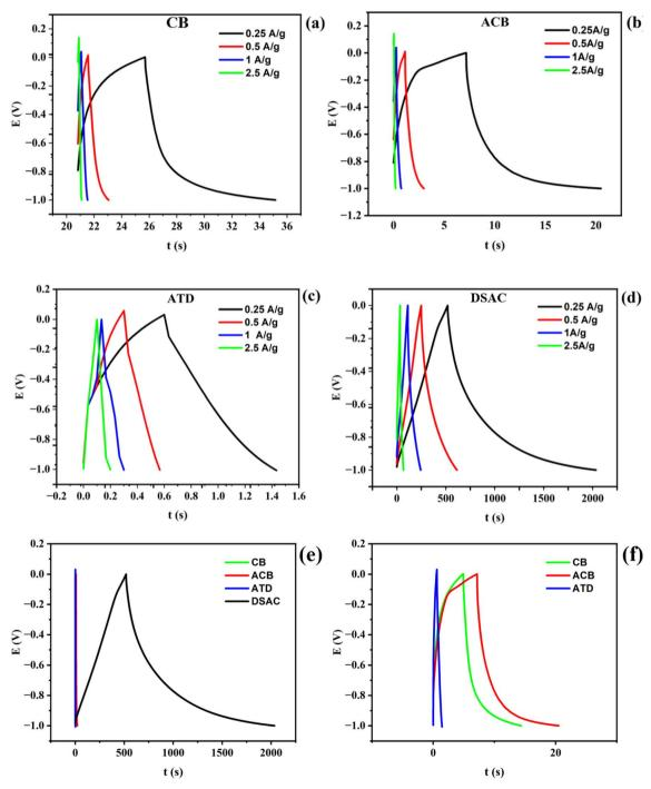
Fig. 8 The galvanostatic charge and discharge cycles of (a) CB, (b) ATD, (c) ACB, and (d) DSAC at scan rates of 0.25 A g<sup>-1</sup>, 0.5 A g<sup>-1</sup>, 1 A g<sup>-1</sup>, and  $2.5 \text{ A g}^{-1}$  within a voltage range of -1 to 0. (e) Overlaid plots for all the electrode materials at a current density of 0.25 A  $\text{g}^{-1}$  within a voltage range of -1 to 0 and (f) expanded version of the combined plot labelled (e) without DSAC.
