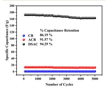
Fig. 9 Cycling stability plot for the CB, ACB, and DSAC electrode samples at a current density of 1 A g<sup>-1</sup>.
