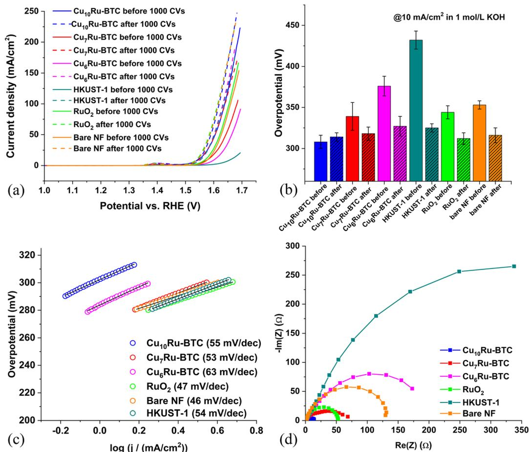
Fig. 6 (a) LSV curves before and after 1000 CVs of Cu<sub>6</sub>Ru-BTC, Cu<sub>7</sub>Ru-BTC, Cu<sub>10</sub>Ru-BTC, HKUST-1, bare NF, and RuO<sub>2</sub>. (b) Overpotentials calculated from LSV curves in (a). (c) Tafel plots for Cu<sub>6</sub>Ru-BTC, Cu<sub>7</sub>Ru-BTC, Cu<sub>10</sub>Ru-BTC, HKUST-1, bare NF, and RuO<sub>2</sub>. (d) Nyquist plots gathered from EIS for Cu<sub>6</sub>Ru-BTC, Cu<sub>7</sub>Ru-BTC, Cu<sub>10</sub>Ru-BTC, HKUST-1, bare NF and RuO<sub>2</sub>.
