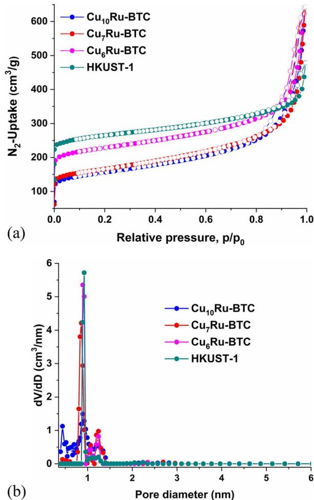
Fig. 4 (a)  $\text{N}_2$ -sorption isotherms at 77 K (adsorption filled circles; desorption empty circles) and (b) NLDFT-derived pore size distributions of  $\text{Cu}_6\text{Ru-BTC}$ ,  $\text{Cu}_7\text{Ru-BTC}$ ,  $\text{Cu}_{10}\text{Ru-BTC}$  and mechanochemically synthesized HKUST-1 (model cylindrical pores at metal oxide).
