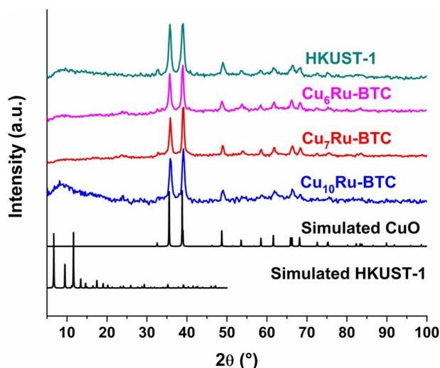
Fig. 8 PXRD patterns of mechanochemically synthesized HKUST-1, Cu<sub>6</sub>Ru-BTC, Cu<sub>7</sub>Ru-BTC, Cu<sub>10</sub>Ru-BTC, following 24 h in 1 mol L<sup>-1</sup> KOH solution, simulated CuO (COD: 15-26990) and simulated HKUST-1 (CCDC no. 112954).
