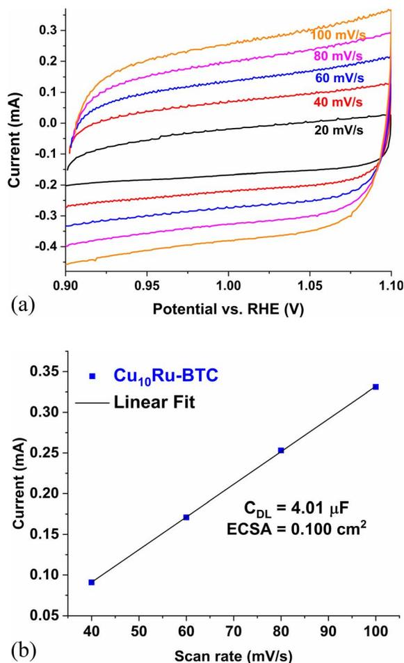
Fig. 7 (a) CV plots of Cu<sub>10</sub>Ru-BTC with different scan rates used for the calculation of the ECSA; (b) current vs. scan rate plot obtained from the CVs in (a) (C<sub>DL</sub> = double layer capacitance, ECSA = electrochemical surface area).
