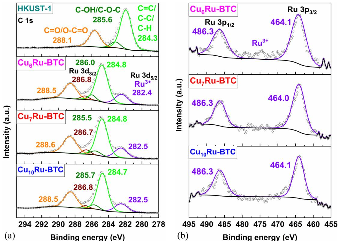
Fig. 5 HR-XPS spectra of (a) C 1s and Ru 3d and (b) Ru 3p for Cu<sub>10</sub>Ru-BTC, Cu<sub>7</sub>Ru-BTC, Cu<sub>6</sub>Ru-BTC and mechanochemically synthesized HKUST-1.
