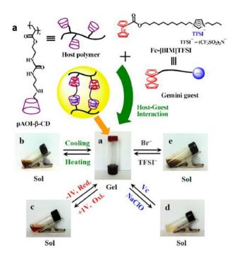
Fig. 46 (a) Preparation of ionic liquid gemini guest cross-linked electroactive supramolecular gels and (b–e) their assembly and disassembly induced by multistimuli. Reproduced from ref. 225 with permission from ACS, Copyright [2014].
