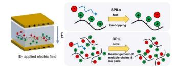
Fig. 68 Schematic illustration of the bulk ion transport in DPILs vs. SPILs. In SPILs, individual ions can move relatively independently of other charged units. However, in DPILs movement of a single ion requires rearrangement of multiple chains and ion pairs. Reproduced from ref. 22 with permission from ACS, Copyright [2021].
