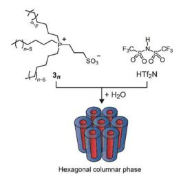
Fig. 14 Zwitterionic compounds 3n consisting of a phosphonium cation and a sulfonate anion. An equimolar mixture of 3n and HTf2N forms a homogeneous complex that exhibits lyotropic columnar liquid crystalline phases in the presence of water. Reproduced from ref. 104 with permission from RSC, Copyright [2011].
