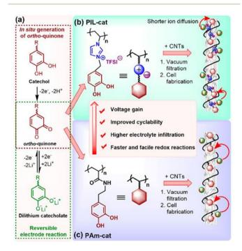
Fig. 32 Construction of catechol-based PIL/CNTs buckypaper for LIBs. (a) ortho-Quinone/dilithium catecholate redox reaction. (b and c) Enhancement in the electrochemical performance of cationic PII -cat (b) compared to its neutral counterpart PAm-cat (c). Reproduced from ref. 212 with permission from ACS, Copyright [2018].
