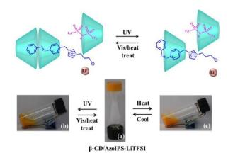
Fig. 47 (a) Mode of inclusion between b-CD and AzolPS-LiTFSI before and after UV irradiation. (b) Preparation of the supramolecular hydrogel: (a) b-CD/AzoIPS-LiTFSI (3:1), and its disassembly induced by: (b) UV light, and (c) temperature. Reproduced from ref. 226 with permission from Wiley-VCH, Copyright [2018].
