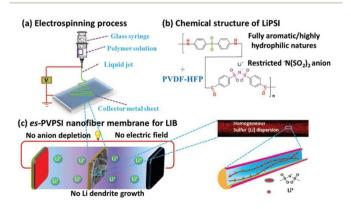
Fig. 33 Schematic illustration of the fabrication (a), composition (b), and operation (c) of the es-PVPSI nanofiber-based membrane, acting as single-ion conducting polymer electrolyte in LIBs. Reproduced from ref. 213 with permission from Wiley-VCH, Copyright [2019].
