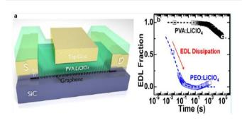
Fig. 65 (a) Schematic representation of the graphene FET fabricated; (b) enhancing the room-temperature electric double layer retention time in 2-D crystal FETs. Reproduced from ref. 251 with permission from ACS, Copyright [2017].
