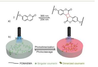
Fig. 55 (a) Reversible dimerization and cleavage of coumarin groups upon exposure to 365/254 nm light. (b) Schematic diagram of crosslinking network formation and dissociation. Reproduced from ref. 235 with permission from BME-PT, Copyright [2023].
