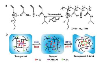
**Fig. 45** (a) Reaction scheme for the preparation of PIL-based membranes *via in situ* photocrosslinking (DVB as the cross-linking agent). (b) Mechanism for thermo-and pH-responsive behaviors. Reproduced from ref. 224 with permission from RSC, Copyright [2016].
