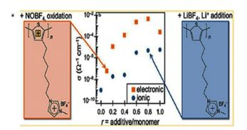
Fig. 39 (a) Schematic structure of the thiophene-based conjugated polymeric ionic liquid used in this study. (b) Electronic conductivity as a function of NOBF<sub>4</sub> oxidant addition. Reproduced from ref. 219 with permission from ACS, Copyright [2021].
