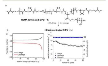
Fig. 31 (a) Schematic representation of the polyurethane-based polymer investigated in the current study. (b) Lithium metal/XSIPU-PC/ LiFePO<sub>4</sub> cell potential versus specific discharge capacity at C/10 and ambient temperature; (c) specific capacity versus cycle number. Reproduced from ref. 211 with permission from Elsevier, Copyright [2017].
