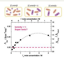
Fig. 5 Molar conductivity ( $\Lambda_{imp}$ ) and ionicity ( $\Lambda_{imp}/\Lambda_{ideal}$ ) of [C<sub>3</sub>mim]I<sup>-</sup> with added  $I_2$  as a function of  $I_3^-$  ( $I^-$ ) concentration at iso-viscosity state of 0.2 Pa s. Reproduced from ref. 65 with permission from RSC, Copyright [2018].
