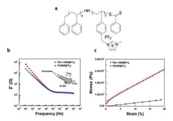
Fig. 26 (a) Schematic representation of the random copolymer-based ionic conductive gel. (b) Resistance (Z') versus frequency (Hz) plots and (c) stress-strain curves for the ion gels composed of 40 wt% P[S-r-VBMI][PF6] or P[VBMI][PF6] and 60 wt% [EMI][TFSI]. The inset of (b) depicts the electrode/ion gel/electrode cell structure used in electrochemical impedance spectroscopy (EIS) experiments. Reproduced from ref. 4 with permission from Wiley-VCH, Copyright [2018].
