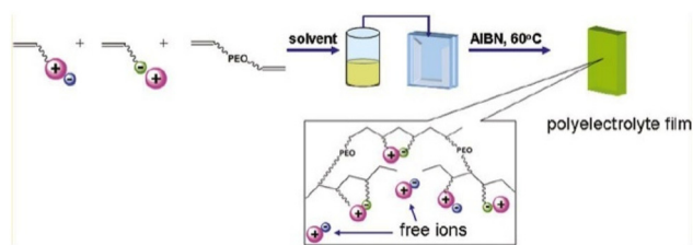
Fig. 63 Schematic representation of the copolymerization of oppositely charged monomers. Reproduced from ref. 12 with permission from ACS, Copyright [2011].
