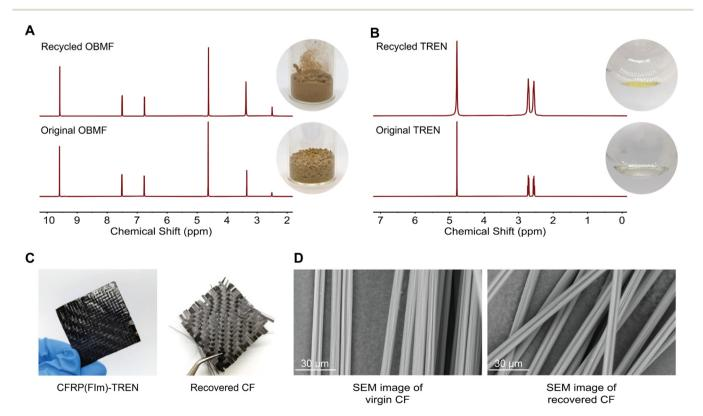
Fig. 2 Chemical recycling of P(FIm)-TREN: physical appearance and <sup>1</sup>H NMR spectra of OBMF in DMSO-d<sub>6</sub> (A) and TREN in D<sub>2</sub>O (B) after depolymerization and subsequent purification, visual appearance of CFRP(FIm-TREN) and recovered carbon fiber cloth upon depolymerization of the composite (C), SEM images of virgin and recovered carbon fibers (D). Scale bar is 30  $\mu m$ .
