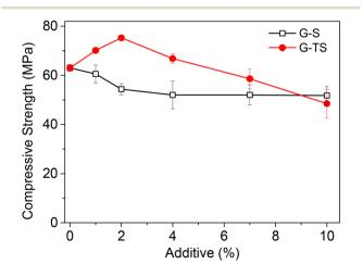
Fig. 4 Compressive strength values of geopolymer and geopolymersawdust composites.
