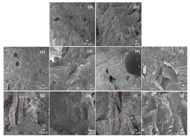
Fig. 3 SEM pictures of geopolymer and geopolymer–sawdust composites at two magnifications (×500 and ×5000). (a) and (b) G, (c) and (d) G-TS2, (e) and (f) G-S2, (g) and (h) G-TS10 and (i) and (i) G-S10.
