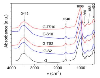
spectra of geopolymer and geopolymer-sawdust Fig. 2 FTIR composites.
