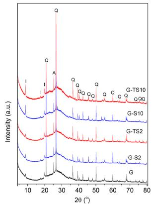
Fig. 1 X-ray patterns of geopolymer and geopolymer-sawdust composites.
