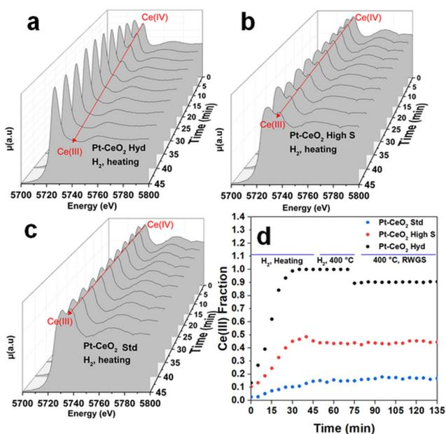
Fig. 4 Time evolution of the *in situ* XANES spectra at the Ce L<sub>3</sub> edge during heating treatment to 400 °C under H<sub>2</sub> atmosphere for a) Pt–CeO<sub>2</sub> Hyd, b) Pt–CeO<sub>2</sub> high S and c) Pt–CeO<sub>2</sub> Std samples. d) Time evolution of the Ce(III) fraction in the Pt–CeO<sub>2</sub> samples during reduction and RWGS reaction.
