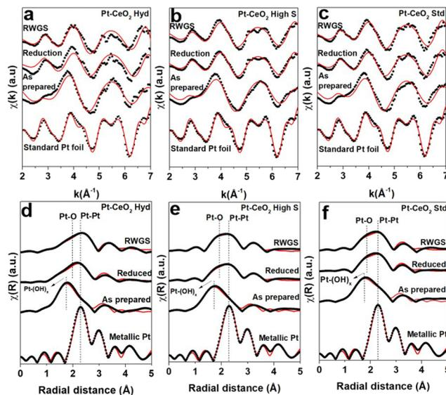
Fig. 5 EXAFS oscillations from *in situ* EXAFS measurements at the Pt L<sub>3</sub> edge of the as-prepared Pt–CeO<sub>2</sub> samples, during reduction treatment and RWGS reaction (a–c) and the respective Fourier transform (d–f). The best fitting found is represented by the red line.
