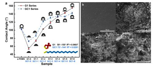
Fig. 10 The (a) contact angle test of the G1 and GC1 e-HMS-PDMS coatings; FSEM images of the (b) EBI crosslinked PDMS and (c-e) G1-3 e-HMS-PDMS coatings.
