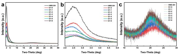
Fig. 3 The XRD patterns of the hybrid materials of the G1 series. (a) 2-40 degrees; (b) 2-5 degrees; (c) 10-30 degrees.
