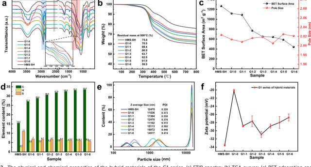
Fig. 2 The physical and chemical properties of the hybrid materials of the G1 series. (a) FTIR spectra; (b) TGA curves; (c) BET adsorption specific surface area and pore size; (d) elemental analysis; (e) particle size distribution curves; (f) zeta potential measurements.
