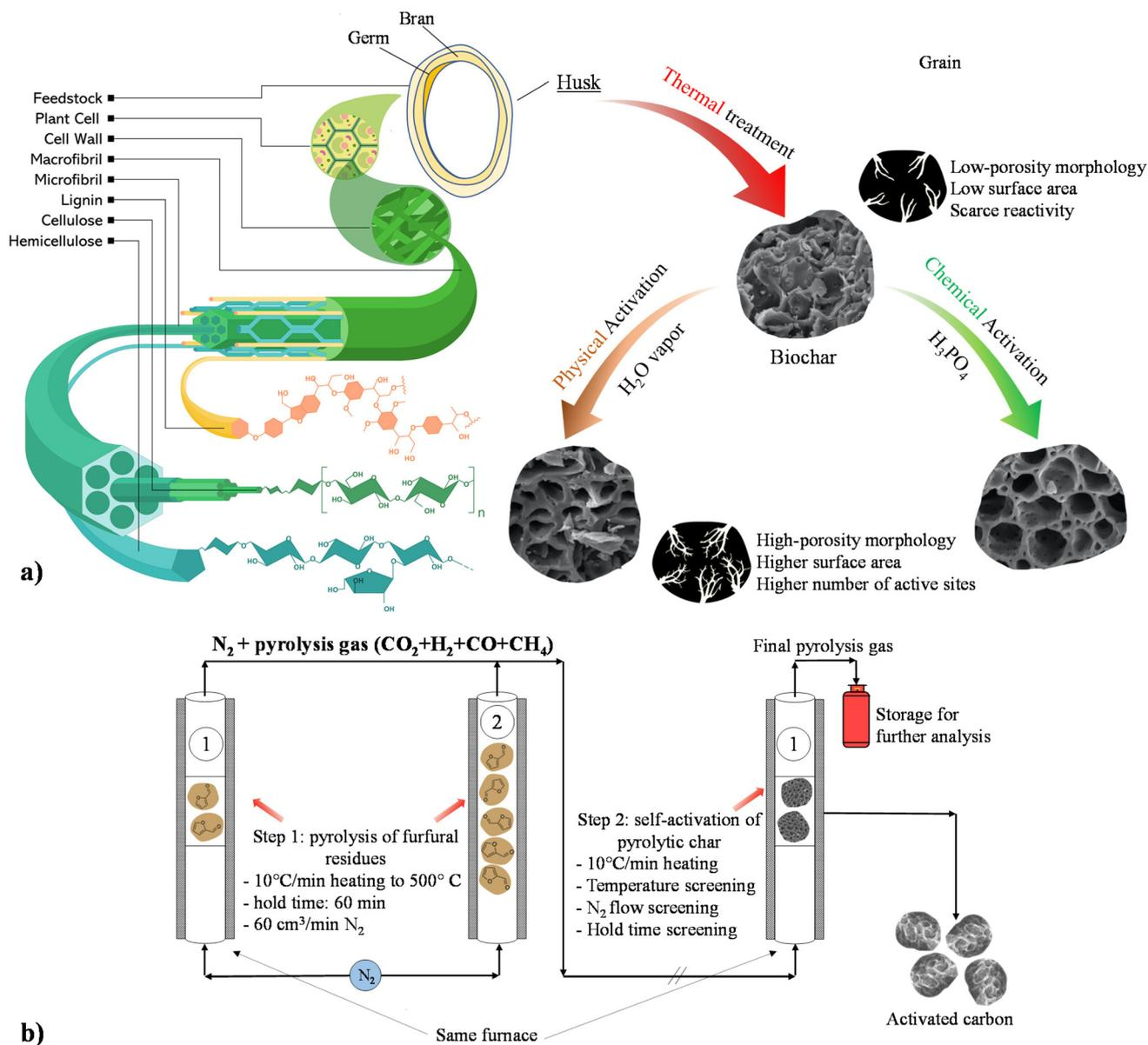
**Fig. 2** (a) AC production from residual biomasses. Reproduced from ref. 86 with permission from Elsevier, Copyright 2021 and from ref. 87 with permission from Wiley, Copyright 2019. (b) Scheme of the AC physical activation process for closed-circle biochar activation. Reproduced from ref. 96 with permission from Elsevier, Copyright 2018.
