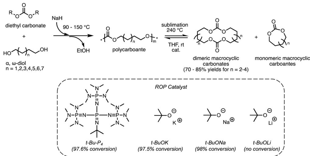
**Scheme 4** Polymerization pathway of polycarbonates from  $\alpha,\omega$ -diol and diethyl carbonate and its recycling via RCD and ED-ROP. Reproduced from ref. 49 with permission from American Chemical Society, copyright 2022.
