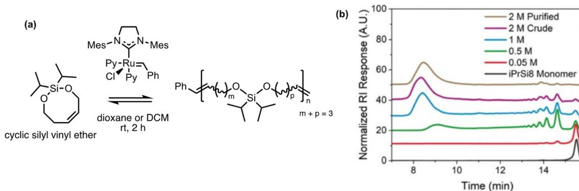
**Fig. 11** Homopolymerization of bifunctional 8-membered silyl ethers via ROMP.<sup>43</sup> (a) Scheme of 8-membered silyl ether forming high molecular weight polysilylether. (b) Size exclusion chromatography of polysilylether prepared at increasing monomer concentration in dioxane. Reproduced from ref. 43 with permission from Royal Society of Chemistry, copyright 2022.
