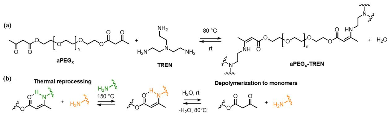
**Scheme 7** (a) Synthesis of the vinylogous urethane network from bis(acetoacetate)-terminated poly(ethylene glycol) (aPEG<sub>x</sub>) and tris(2-aminoethyl) amine (TREN) as the crosslinker. (b) Transamination between an amine and a vinylogous urethane (left) and the reversible hydrolytic depolymerization to the parent monomers (right). Reproduced from ref. 185 with permission from Wiley, copyright 2023.
