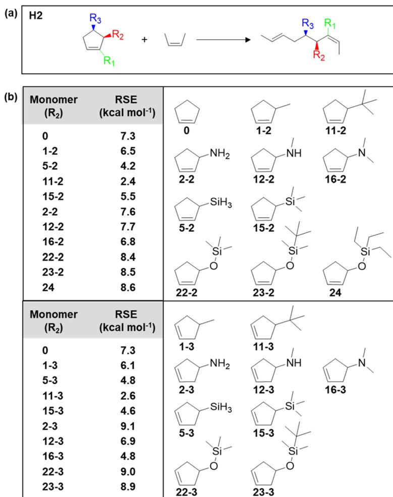
**Fig. 7** (a) Homodesmotic equations used to calculate RSEs. Substituent locations (R) are denoted as alkenyl (R<sub>1</sub>), allylic (R<sub>2</sub>), or homoallylic (R<sub>3</sub>). (b) Calculated RSEs of allylic (R<sub>2</sub>) and homoallylic (R<sub>3</sub>) monomers. The monomer structures correspond to the monomer RSEs in the table. Reproduced from ref. 92 with permission from American Chemical Society, copyright 2023.
