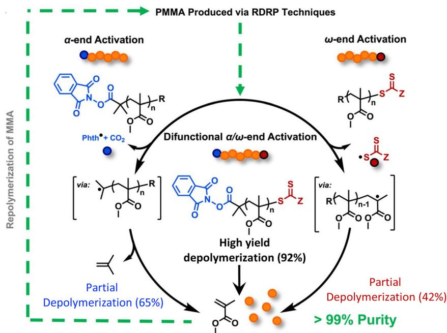
Fig. 13 A scheme depicting the chemical recycling of PMMA to MMA *via* activation of the  $\alpha$ -chain ends,  $\omega$ -chain ends, or a combination of both. Reproduced from ref. 150 with permission from Elsevier, copyright 2023.
