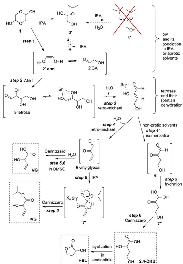
**Scheme 12** Reaction pathway for the conversion of glycolaldehyde in isopropyl alcohol or nonprotic solvents in the presence of homogeneous tin chlorides. Reproduced from ref. 128 with permission from The American Chemical Society, copyright 2013.
