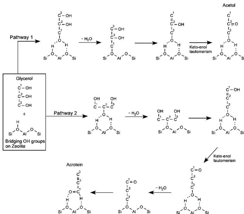
**Scheme 6** Proposed reaction pathways for the conversion of glycerol catalyzed by acid zeolites. Adapted from ref. 90 with permission from Elsevier, copyright 2009.
