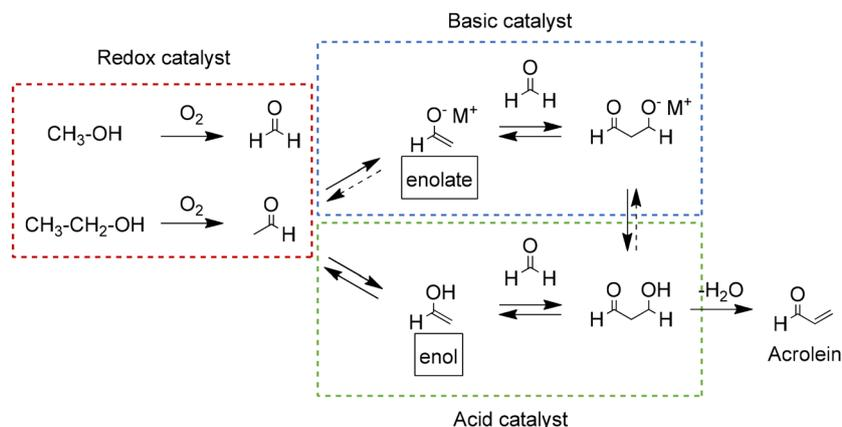
**Scheme 7** Proposed reaction pathways for the catalytic conversion of methanol and ethanol to acrolein. Adapted from ref. 95 with permission from The Royal Society of Chemistry, copyright 2017.
