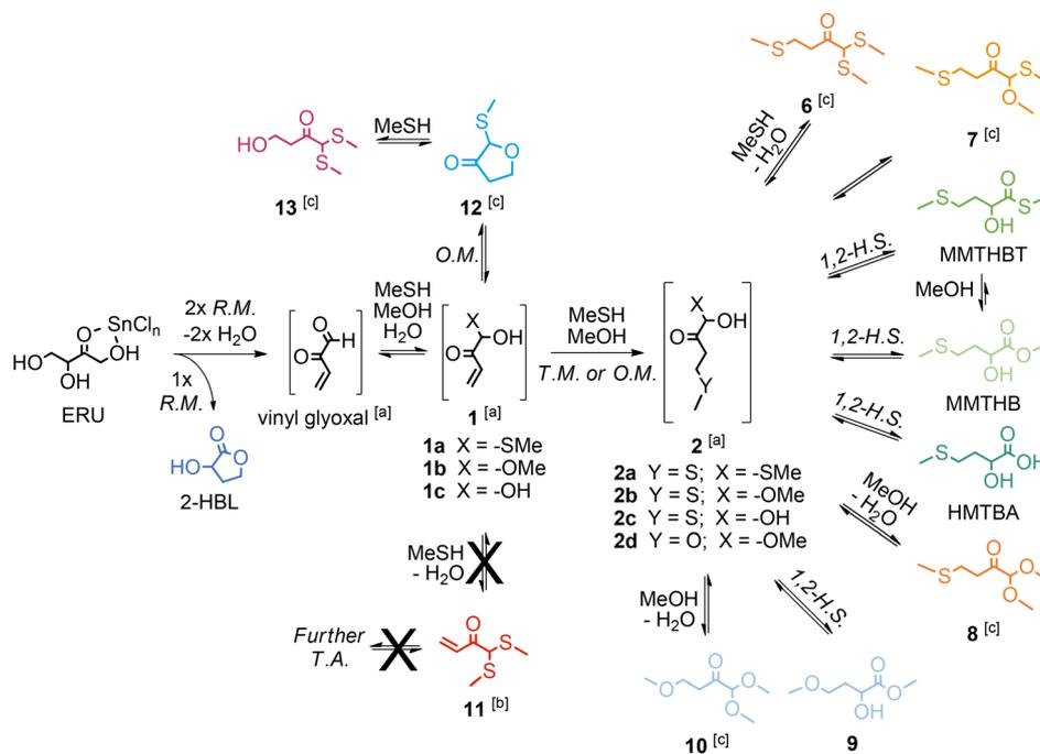
**Scheme 15** Reaction pathways for the conversion of tetroses to methionine hydroxy analogues in the presence of  $\text{Sn}^{\text{IV}}$  Lewis acid catalyst in MeSH/MeOH mixtures. Adapted from ref. 137 with permission from Elsevier, copyright 2023.
