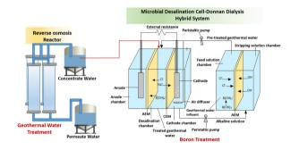
Concurrent boron removal from reverse osmosis concentrate and energy production using a microbial desalination cell-Donnan dialysis hybrid system
