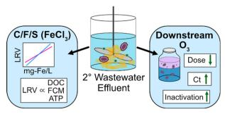
Improved microbial water quality and ozone performance following coagulation: implications for carbon based advanced treatment for potable reuse
