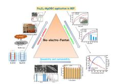
Sludge-derived novel Fe<sub>3</sub>O<sub>4</sub>-MgO@C composites for tetracycline abatement from wastewater using sustainable bio-electro-Fenton and nutrient recovery with co-precipitation; a waste-to-resource strategy
