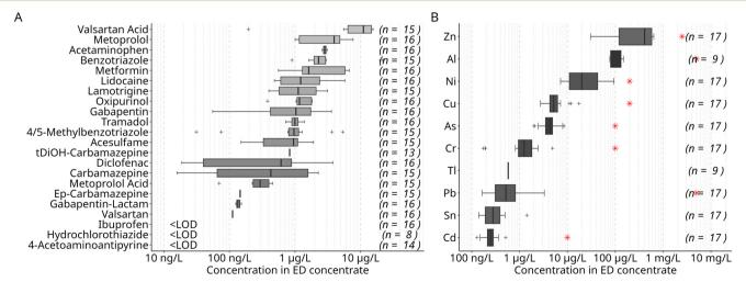
Fig. 6 Concentration of organic micropollutants (A) and metals and metalloids (B) in the electrodialysis concentrate derived as multi-nutrient solution by the nutrient recovery process (n = number of detects in 16 (A) and 17 (B) samples). Red crosses indicate the maximum concentration of metals and metalloids recommended for wastewater reuse.<sup>27</sup>
