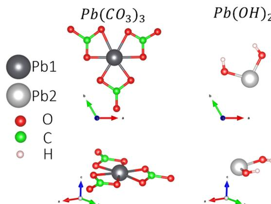
Fig. 2 Atomistic models of the hydrocerussite constituents.
