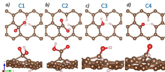
Fig. 1 Top and side views of the four GO atomic models. a) C1, b) C2, c) C3, and d) C4. Brown, red, and white spheres represent C, O, and H atoms.
