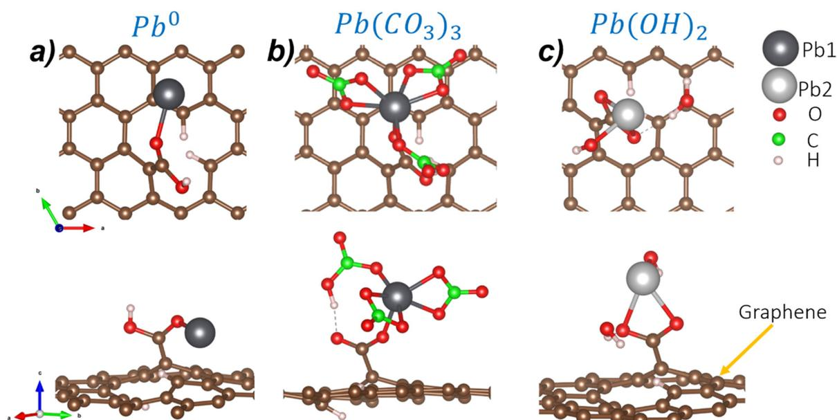
**Fig. 3** The most stable adsorption configurations for a)  $\text{Pb}^0$ , b)  $\text{Pb}(\text{CO}_3)_3$ , and c)  $\text{Pb}(\text{OH})_2$  molecules.
