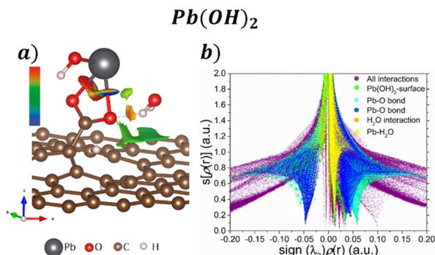
Fig. 6 a) NCI isosurface with  $s = 0.05$  a.u. and b)  $s[\rho(r)]$  vs.  $\text{sign}(\lambda_2)\rho(r)$  graph for the adsorption Pb(OH)<sub>2</sub> on the GO surface.
