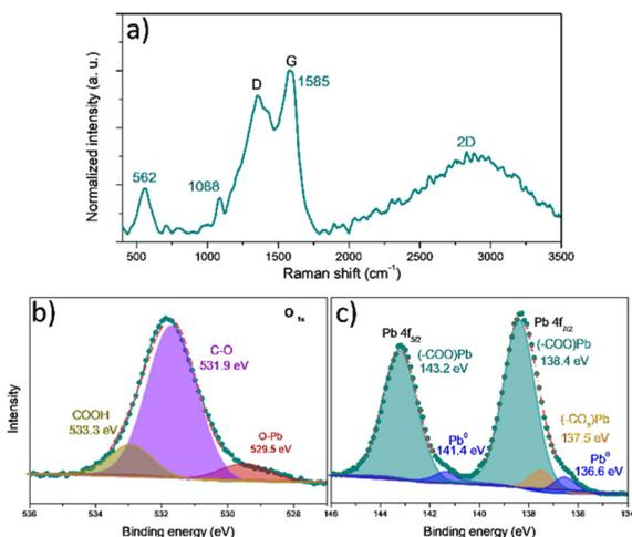
Fig. 7 Experimental characterization of GO-Pb<sup>2+</sup>: a) Raman, b) O 1s, and c) Pb 4f high-resolution XPS spectra.
