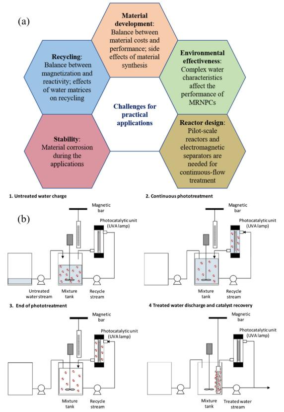
Fig. 8 (a) Challenges of MNRPCs in practical applications; (b) operation of magnetic photocatalytic reactor: 1) loading of MNRPCs and water, 2) continuous phototreatment; 3) end of phototreatment, 4) MNRPCs recycling. Reproduced from ref. 70 with permission from Elsevier, copyright 2019.
