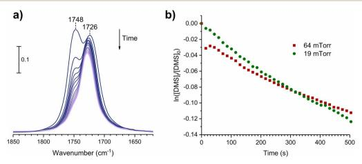
Fig. 5 (a) Temporal desorption FTIR spectra during a 1 h evacuation after the SiO<sub>2</sub> surface was exposed to DMS at 64 mTorr for 30 min. (b) Firstorder desorption kinetics of DMS from SiO<sub>2</sub> surfaces following their exposures at 19 and 64 mTorr.
