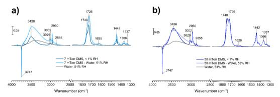
Fig. 8 FTIR spectra of the  $SiO_2$  surface after DMS exposure at an equilibrium pressure of (a) 7 mTorr and (b) 50 mTorr followed by exposure to water vapor at 50  $\pm$  3% RH.
