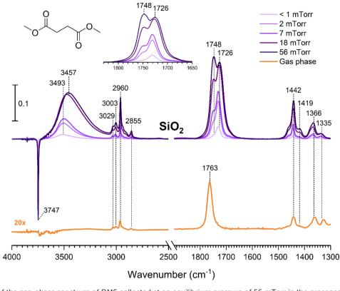
Fig. 1 FTIR spectra of the gas-phase spectrum of DMS collected at an equilibrium pressure of 56 mTorr in the presence of  $SiO_2$  and the  $SiO_2$  surface after DMS exposure at different equilibrium pressures. The 1650 to 1830 cm<sup>-1</sup> region is expanded in the inset to show the evolution of the carbonyl bands more clearly.
