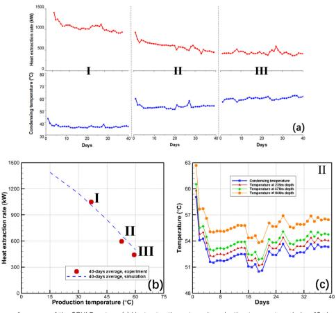
Fig. 4 Heat extraction performance of the SGHLP system. (a) Heat extraction rate and production temperature during 40-day heat extraction tests; (b) comparison of 40-day average heat extraction rates between experimental data and simulation results; (c) SLGHP temperatures measured at three monitoring points underground, i.e., at 235 m, 470 m, and 940 m subsurface, respectively, under the conditions of test II.
