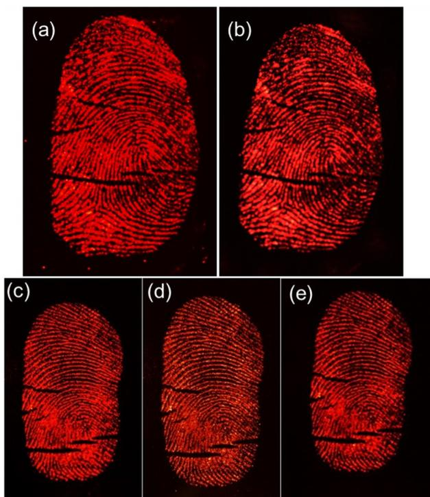
**Fig. 14** Photographs for the visualization of LFPs developed on a silicon wafer surface using the  $\text{Eu}_{0.1}\text{-BAO-900}$  nanophosphor observed under a 254 nm mercury-vapour UV lamp with aging times of 1 (a) and (b) 40 days for the right thumb and (c) 1, (d) 40 and (e) 60 days for the left thumb of the same volunteer in ambient atmosphere.
