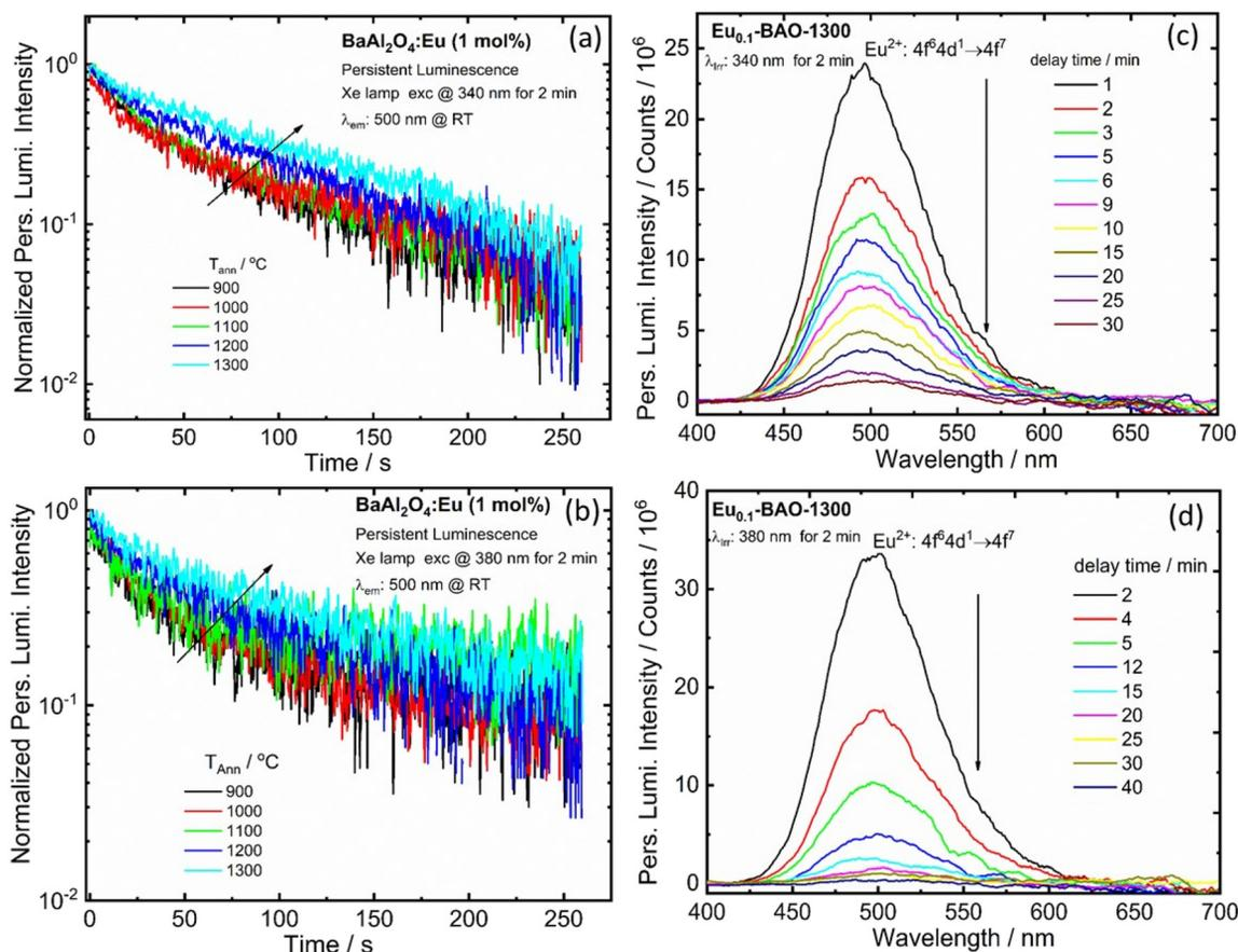
Fig. 7 Persistent luminescence decay time curves (a and b) of the  $\text{Eu}_{0.1}\text{-BAO}$  sample annealed at various temperatures. Persistent luminescence emission spectra (c and d) for the optimum sample ( $\text{Eu}_{0.1}\text{-BAO-1300}$ ), recorded under the same conditions.
