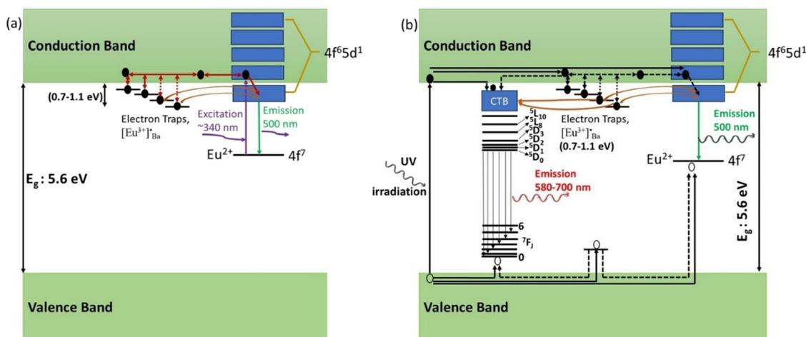
Fig. 12 (a) Proposed persistent luminescence mechanism of  $\text{BaAl}_2\text{O}_4\text{:Eu}^{2+}/\text{Eu}^{3+}$  in the case of low energy UV excitation ( $\sim 340$  nm) and (b) the electron trapping–detrapping persistent luminescence mechanism in the case of band-to-band excitation (254 nm).
