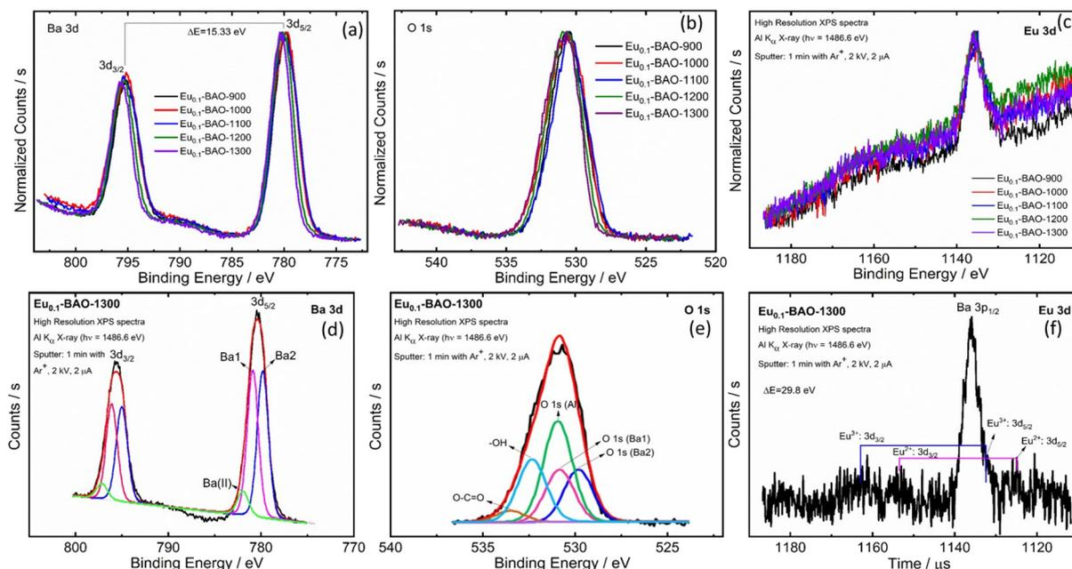
Fig. 3 High resolution XPS spectra of  $\text{Eu}_{0.1}\text{-BAO}$  phosphors: (a) Ba 3d, (b) O 1s and (c) Eu 3d and the peak fits for (d) Ba 3d, (e) O 1s and (f) Eu 3d for the  $\text{Eu}_{0.1}\text{-BAO-1300}$  sample.
