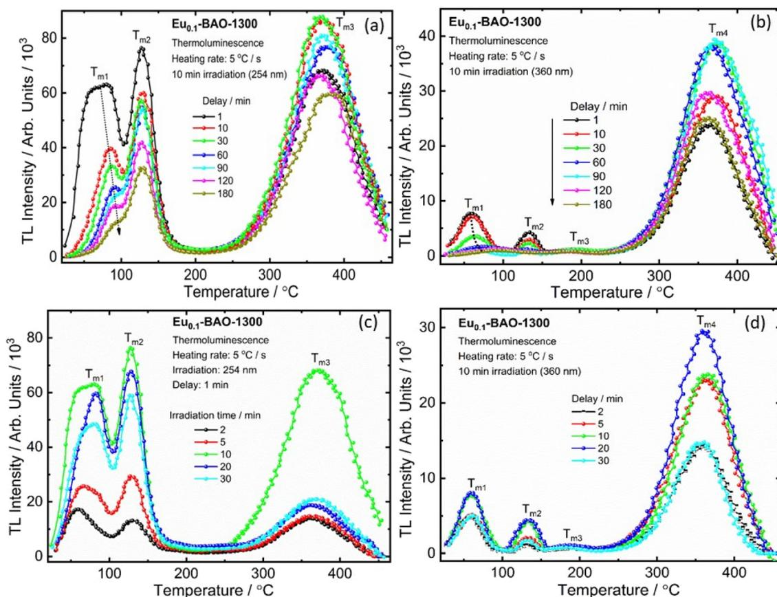
**Fig. 11** Thermoluminescence glow curve of the Eu<sub>0.1</sub>-BAO-1300 phosphor. TL curves of the Eu<sub>0.1</sub>-BAO-1300 phosphor with different delay times from 1 to 180 min (a and b). The phosphors were pre-irradiated with a 254 nm (a) and a 360 nm (b) UV lamp for 10 min. The TL glow curve obtained by irradiating a Eu<sub>0.1</sub>-BAO-1300 phosphor with 254 nm (c) and 360 nm (d) UV lamp for various durations ranging from 2 to 30 minutes.
