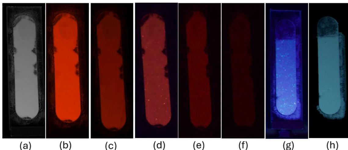
**Fig. 9** Photographic images of the  $\text{Eu}_{0.1}\text{-BAO-1300}$  sample: (a) under a fluorescent lamp; (b) under a 254 nm UV lamp; for 30 s (c), 1 min (d), 2 min (e), and 3 min (f) after removal of the 254 nm UV lamp irradiation at RT; (g) under a 360 nm UV lamp; and (h) 1 min after removal of the 360 nm UV lamp irradiation at RT.
