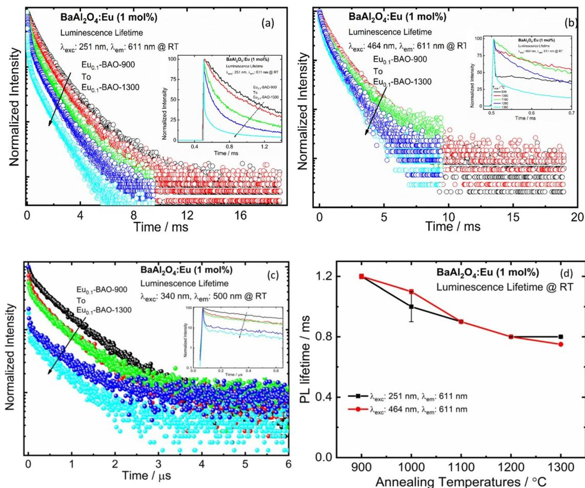
Fig. 6 PL decay curves of the Eu<sub>0.1</sub>-BAO-*x* (*x* = 900–1300) phosphors under excitation at 251 nm (a), 464 nm (b) (*i.e.* Eu<sup>3+</sup>) and 340 nm (c) (*i.e.* Eu<sup>2+</sup>) by monitoring the emission at 611 nm and 500 nm, respectively. (d) Variation graph of PL lifetime with different annealing temperatures.
