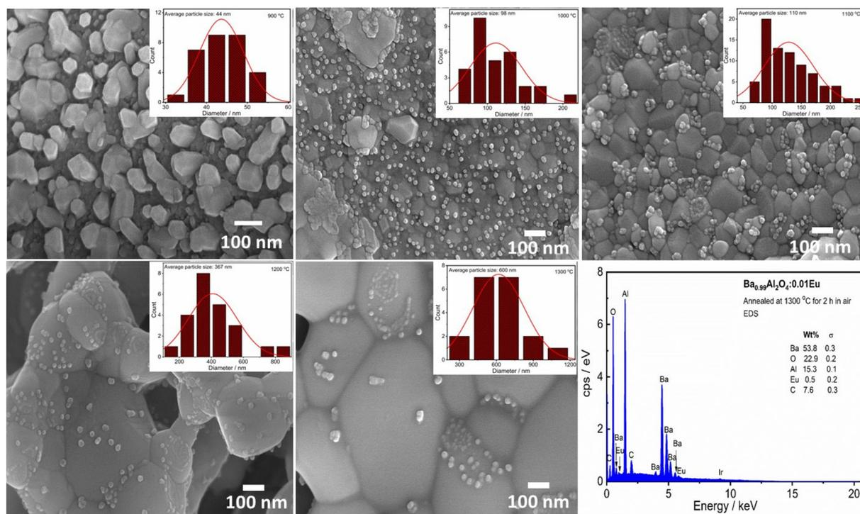
Fig. 2 FE-SEM images of  $\text{Eu}_{0.1}\text{-BAO-}x$  ( $x = 900$  to  $1300$ ) phosphors. The inset shows the size distribution diagrams of  $\text{Eu}_{0.1}\text{-BAO-}x$  ( $x = 900\text{--}1300$ ) phosphors (extracted from FE-SEM images) and the EDS spectrum of the  $\text{Eu}_{0.1}\text{-BAO-}1300$  phosphor.
