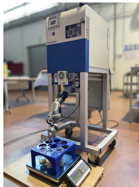
Fig. 7 Final assembly of the pellet distributor, mounted on the pelletizer and filling a tray with several cups on top of a balance for feedback. An air ionizer is mounted at the top of the pellet distributor.
