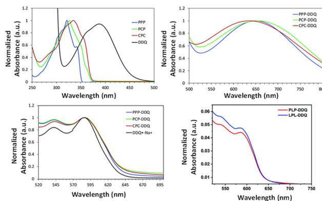
**Fig. 14** Normalized UV-vis absorption spectra of (a) trimers and DDQ in chloroform, (b) charge transfer peak shown for clarity, (c) charge-transfer complexes in tetrahydrofuran and (d) non-normalized spectra of PLP-DDQ and LPL-DDQ complexes in tetrahydrofuran. Reproduced with permission from ref. 26 under a Creative Commons Attribution-Non-commercial 3.0 Unported Licence. Royal Society of Chemistry (2022).
