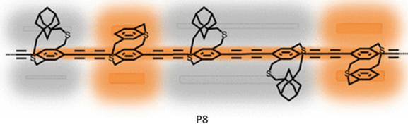
**Fig. 15** Chemical structure of the **P8** polymer containing both adamantyl strapped and *p*-CP comonomers. Randomly positioned *p*-CP units along the insulated polymer backbone enhance the photoinduced charge transfer to acceptor molecules resulting in fluorescence quenching. Reproduced with permission from ref. 65 Copyright American Chemical Society (2021).
