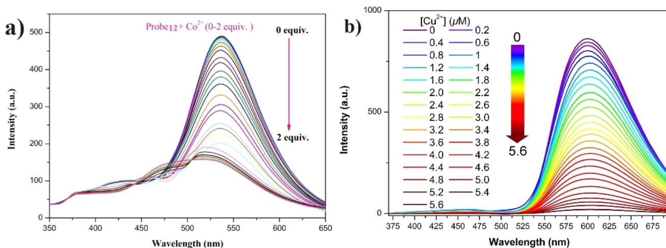
Fig. 18 (a) Emission spectra of probe **12** upon increasing concentrations of  $\text{Co}^{2+}$  ions in THF/ $\text{H}_2\text{O}$  mixtures ( $f_w = 60\%$ ,  $\text{pH} = 7.4$ ,  $\lambda_{\text{ex}} = 330 \text{ nm}$ ). (b) Emission spectra of probe **13** with increasing  $\text{Cu}^{2+}$  ions concentration in THF/ $\text{H}_2\text{O}$  ( $f_w = 90\%$ ,  $\text{pH} = 7.4$ ,  $\lambda_{\text{ex}} = 350 \text{ nm}$ ). Reproduced with permission from ref. 57. Copyright 2023 Springer.
