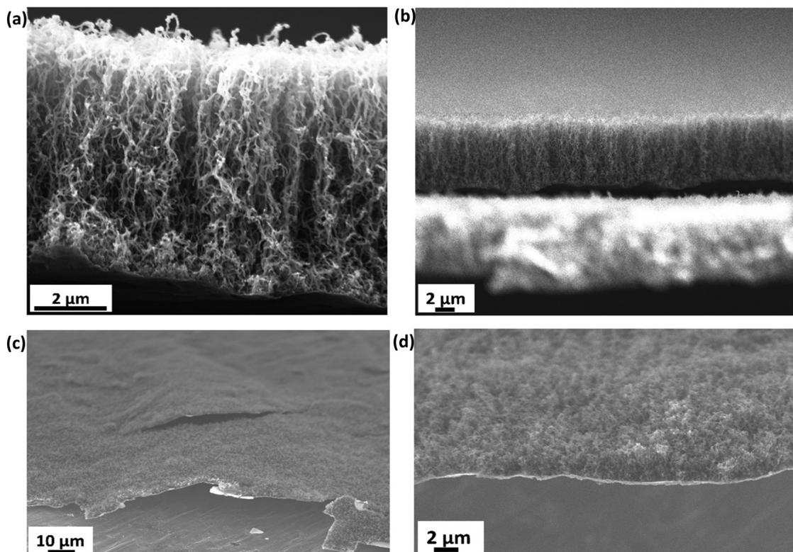
Fig. 2 SEM images representing (a) 7–8  $\mu\text{m}$  thick vertically aligned CNTs on Cu after 30 min CVD growth. (b) Zoomed out picture of panel (a) showing uniformity in thickness of the CNTs. (c) Poor adhesion of CNTs to the substrate after prolonged growth time and (d) tilted image showing forest-like growth.
