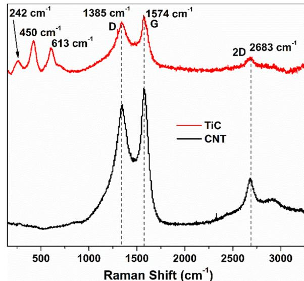
Fig. 3 Raman spectra collected from two samples at a laser excitation wavelength of 532 nm: (black) standard CNT/Fe/Al<sub>2</sub>O<sub>3</sub>/Cu sample where CNTs were grown by CVD and (red) the sample without the Fe catalyst resulting in no CNT growth but verifying the presence of the TiC interface.
