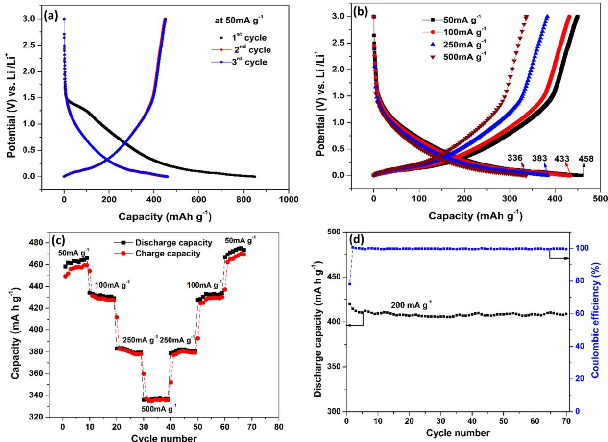
Fig. 5 Galvanostatic charge discharge profiles of CNTs on the Cu substrate. (a) First three charge–discharge cycles at 50 mA g<sup>-1</sup>. (b) Electrode subjected to various current densities from 50–500 mA g<sup>-1</sup>. (c) High-rate cycling performance. (d) Discharge capacity and coulombic efficiency vs. cycle number at the current density of 200 mA g<sup>-1</sup>.
