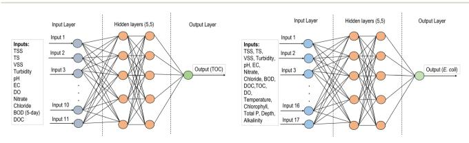
Fig. 2 ANN model architecture for TOC prediction (left) and E. coli prediction (right).
