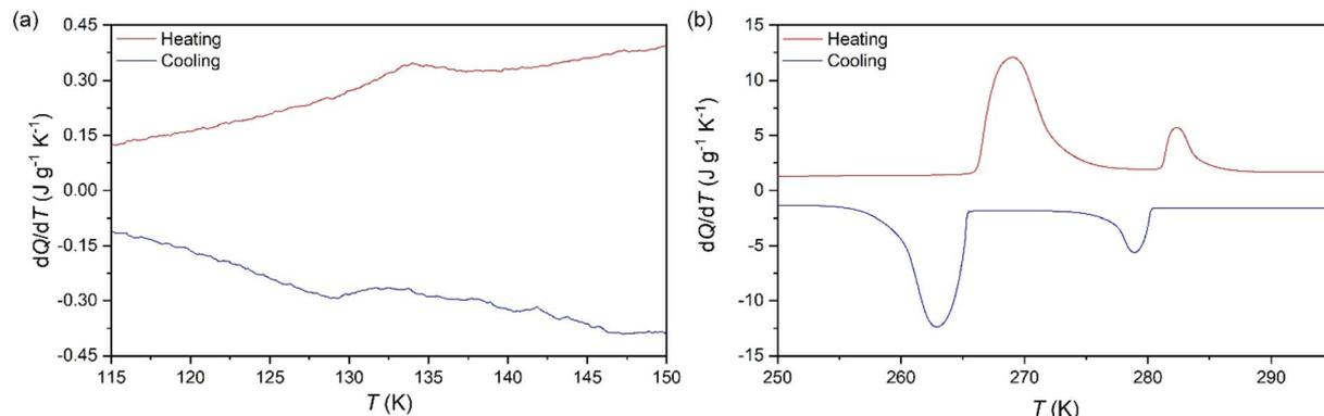
Fig. 1 VT-DSC curves for the [DBA][BF<sub>4</sub>] compound in the (a) lower- and (b) higher-temperature ranges.
