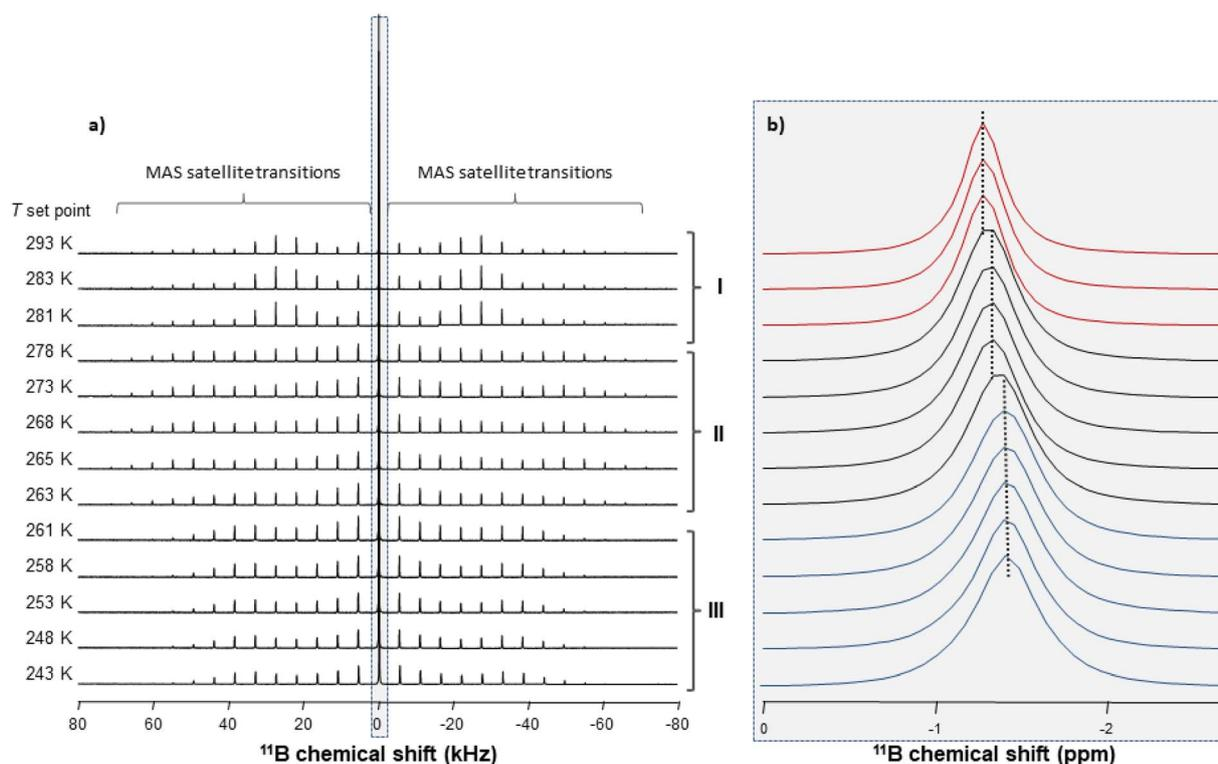
Fig. 13  $^{11}\text{B}$  MAS NMR spectra obtained at different temperatures ( $\nu_0 = 193$  MHz and  $\nu_{\text{MAS}} = 5.5$  kHz): (a) full spectral window showing the MAS satellite transition sidebands; (b) zoomed-in view of the isotropic centre band.
