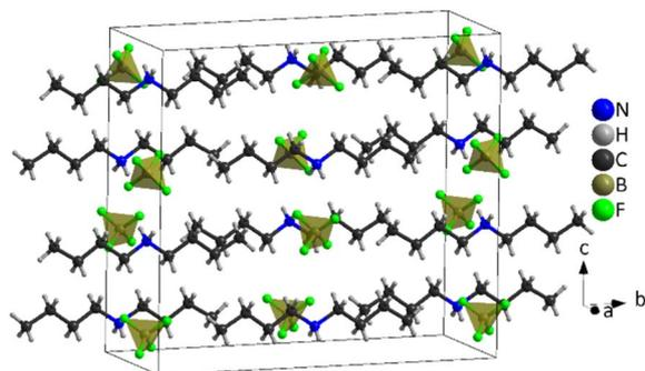
Fig. 7 Structure of [DBA][BF<sub>4</sub>] at 100 K (PIV), where the tetrahedra correspond to [BF<sub>4</sub>]<sup>-</sup> anions and the chains to [DBA]<sup>+</sup> cations and the black cage represents the unit cell.
