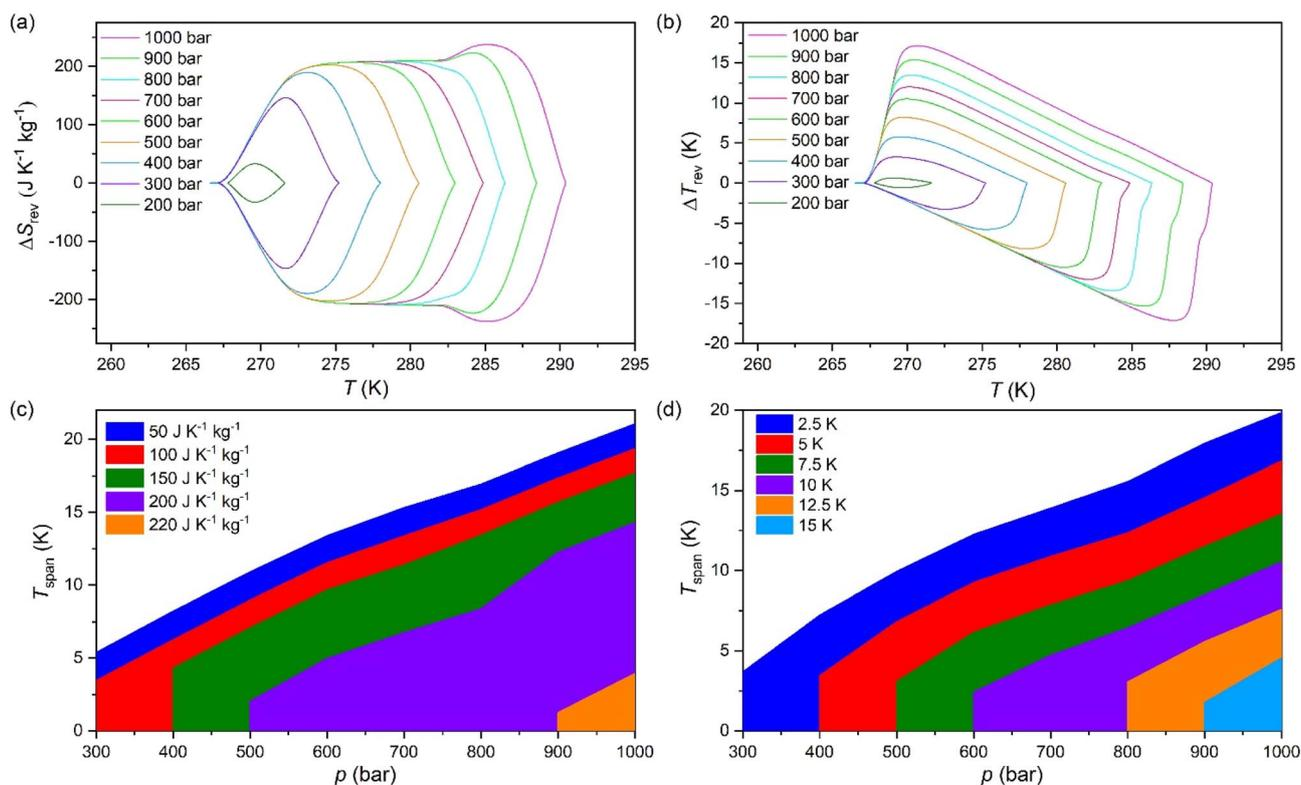
Fig. 4 (a) Pressure-driven reversible isothermal entropy changes on applying ( $0 \rightarrow p$ ) and removing ( $p \rightarrow 0$ ) pressure. (b) Reversible adiabatic temperature changes on applying ( $0 \rightarrow p$ ) and removing ( $p \rightarrow 0$ ) pressure at different pressures. (c) Temperature span as a function of applied pressure for fixed intervals of reversible isothermal entropy changes and (d) reversible adiabatic temperature changes for [DBA][BF<sub>4</sub>].
