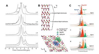
Fig. 5 (A) Solid-state <sup>1</sup>H NMR spectra of Mg/Al-2-LDH. (B) Schematic illustration of Mg/Al-2-LDH. (C) Quantitative fitting of the <sup>1</sup>H echo-MAS NMR spectra of LDH.81 Copyright © 2011 American Chemical Society.
