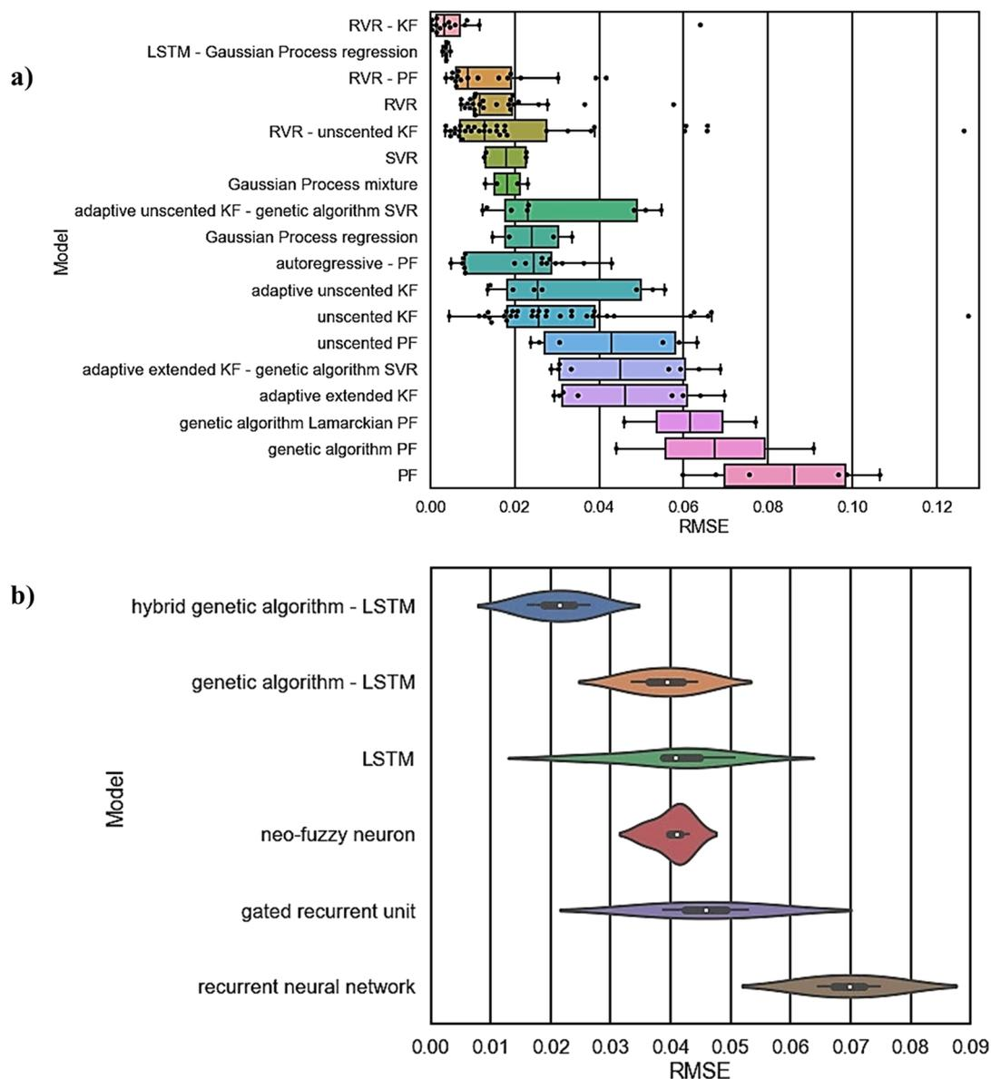
Fig. 20 (a) Boxplots of various models' RMSE for RUL prediction of LIBs (RVR = relevance vector regression, PF = particle filter, KF = Kalman filter, SVR = support vector regression).<sup>187–189,206–212</sup> (b) Violin plots of various models' RMSE for RUL prediction of supercapacitors (LSTM = long-short term memory).<sup>190,191,213</sup>
