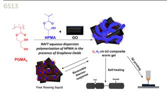
3D printable, thermo-responsive, self-healing, graphene oxide containing self-assembled hydrogels formed from block copolymer wormlike micelles
