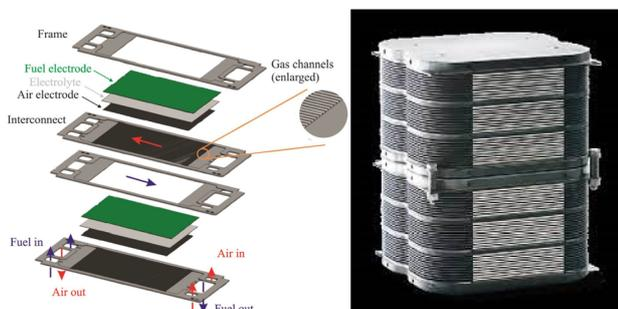
Fig. 16 Sunfire solid oxide cell and stack technology for co-SOE electrolysis (Masini *et al.*, 2019; Sunfire, 2022).<sup>69,70</sup>
