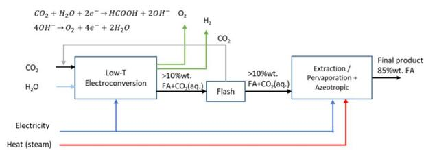
Fig. 7 Process diagram of the LT CO<sub>2</sub> electrolysis towards FA.
