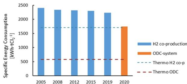
Fig. 3 Evolution of the specific energy consumption for the production of Cl<sub>2</sub> through the membrane electrolysis technology since 2005. H<sub>2</sub> co-production is the conventional technology seen in Fig. 2 and the oxygen depolarised cathode (ODC) technology represents a novel design in which oxygen is used at the cathode. Plot constructed with data from ref. 14 and 17.
