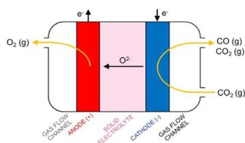
Fig. 12 Principle of CO production in a solid oxide cell (Küngas, 2020).<sup>30</sup>
