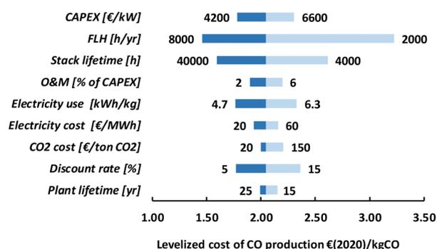
Fig. 24 Sensitivity analysis for route 4 – HT electrochemical conversion of CO<sub>2</sub> to CO. Nine parameters are varied to explore their effect on the current levelized cost of CO production. The fossil reference CO price amounts to 0.07–0.18€ per kg<sub>CO</sub>.
