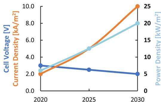
Fig. 6 Roadmap for different process performance indicators for LT CO<sub>2</sub> electrolysis for the current decade. Considered products are CO, FA, and C<sub>2</sub>H<sub>4</sub>. Reproduced from ref. 28.
