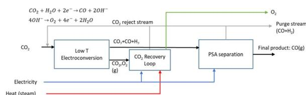
Fig. 4 Process diagram of the LT CO<sub>2</sub> electrolysis towards CO.
