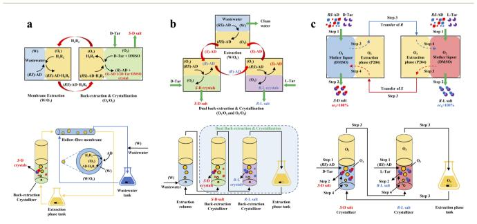
Fig. 2 Mechanisms and schematic diagrams of (a) extraction-crystallization-membrane coupling method,<sup>51</sup> (b) multiple-phase extraction and *in situ* coupling of crystallization,<sup>52</sup> and (c) pairwise crystallization-circulating extraction coupling method for mother liquor *in situ* reuse.<sup>147</sup>
