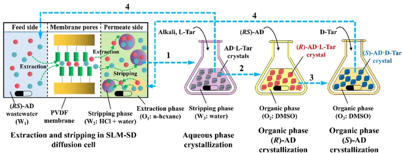
Fig. 32 Schematic diagram of the integrated supported liquid membrane-organic/organic phase crystallization separation process (step 1: transfer of  $W_2$  from SLM-SD, step 2: transfer of aqueous phase crystal from  $W_3$ , step 3: transfer of the mother liquor from  $O_2$ , and step 4: mother liquor recycling routes of  $O_3 \rightarrow O_1$  and  $W_3 \rightarrow W_1$ ).<sup>341</sup>
