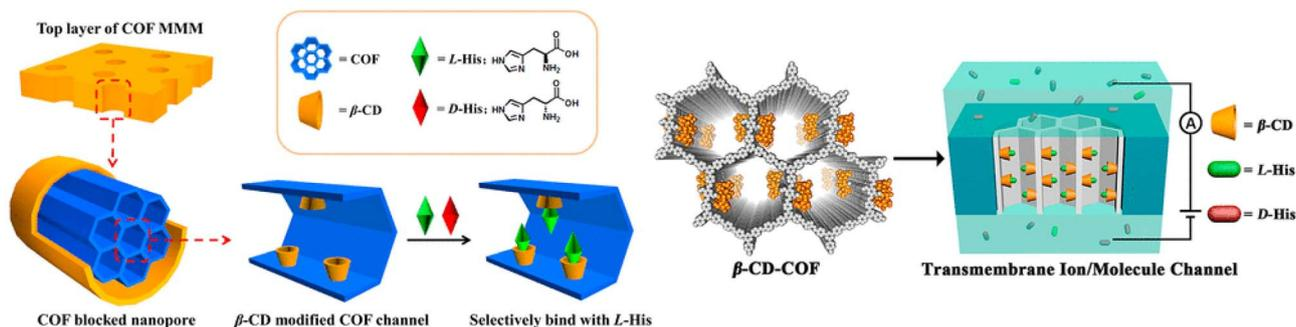
Fig. 28 Schematic representation of the construction of  $\beta$ -CD-COF MMMs and subsequent voltage-driven enantioselective transport.<sup>333</sup> Reproduced with permission from ref. 333. Copyright 2019, the American Chemical Society.
