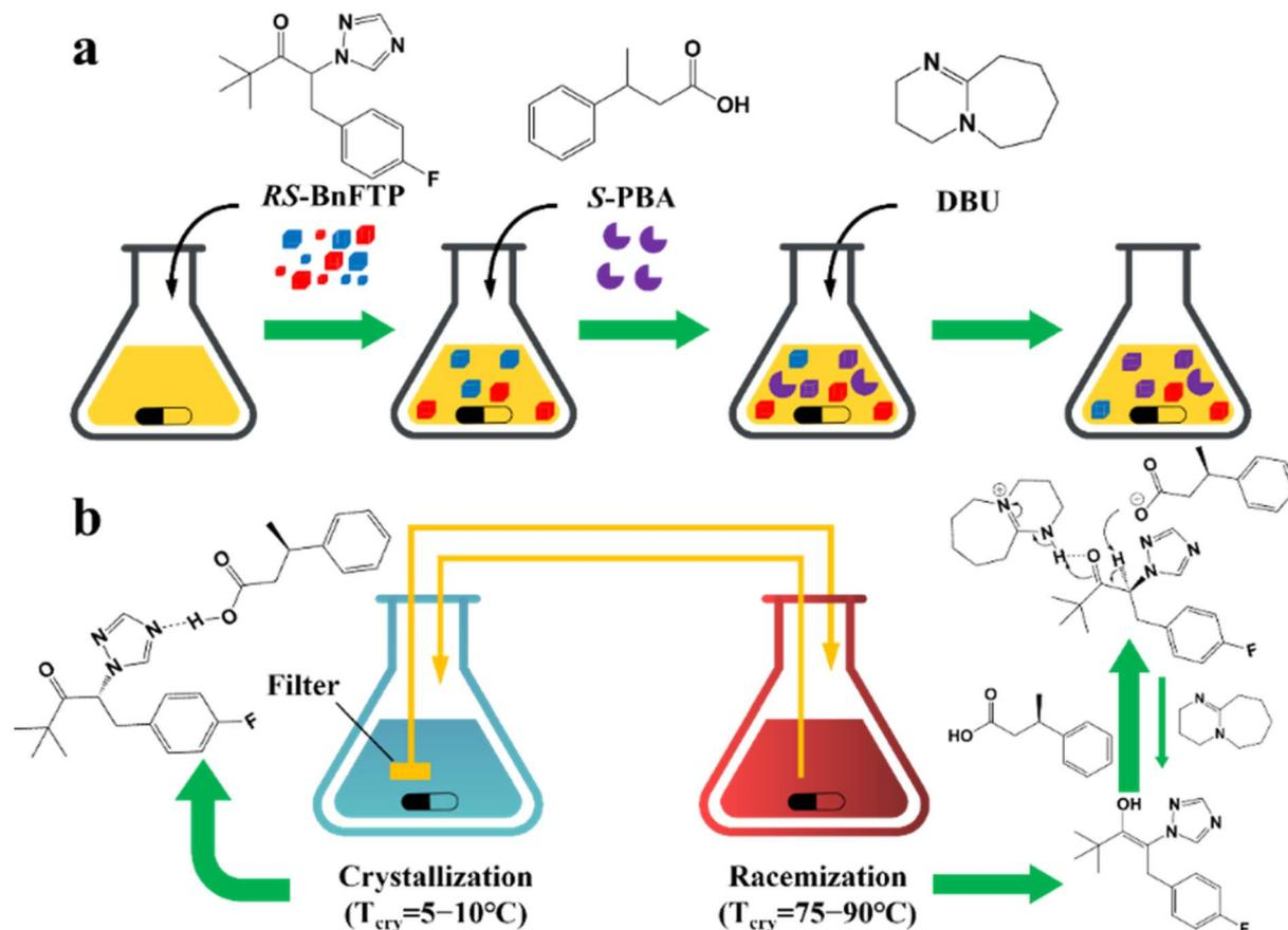
Fig. 13 (a) Schematic representation of the CoISD process and (b) the CoISD mechanism that occurred in a two-vessel setup with the cocrystal in suspension.<sup>55,239</sup> *RS*-BnFTP, PBA and DBU represent the racemic mixture, chiral coformer and racemizing agent, respectively.
