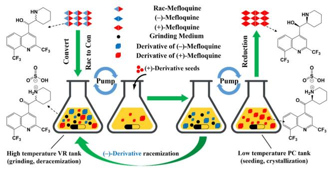
Fig. 17 Experimental chemical derivatization-VR-PC coupled setup used for the deracemization of mefloquine.<sup>262</sup> Blue arrows: crystal-free liquid exchange through tubes.
