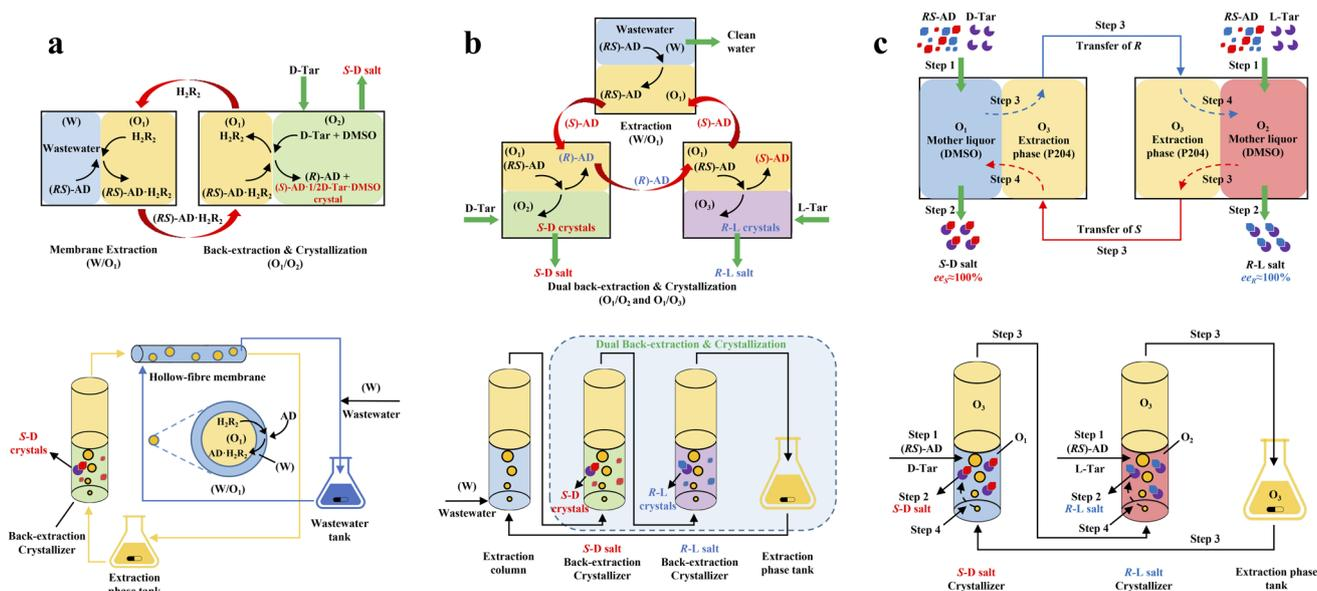
Fig. 2 Mechanisms and schematic diagrams of (a) extraction-crystallization-membrane coupling method,<sup>51</sup> (b) multiple-phase extraction and *in situ* coupling of crystallization,<sup>52</sup> and (c) pairwise crystallization-circulating extraction coupling method for mother liquor *in situ* reuse.<sup>147</sup>
