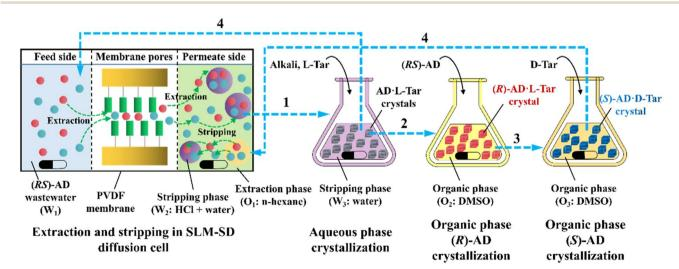
Fig. 32 Schematic diagram of the integrated supported liquid membrane-aqueous/organic phase crystallization separation process (step 1: transfer of W<sub>2</sub> from SLM-SD, step 2: transfer of aqueous phase crystal from W<sub>3</sub>, step 3: transfer of the mother liquor from O<sub>2</sub>, and step 4: mother liquor recycling routes of O<sub>3</sub>  $\rightarrow$  O<sub>1</sub> and W<sub>3</sub>  $\rightarrow$  W<sub>1</sub>).<sup>341</sup>
