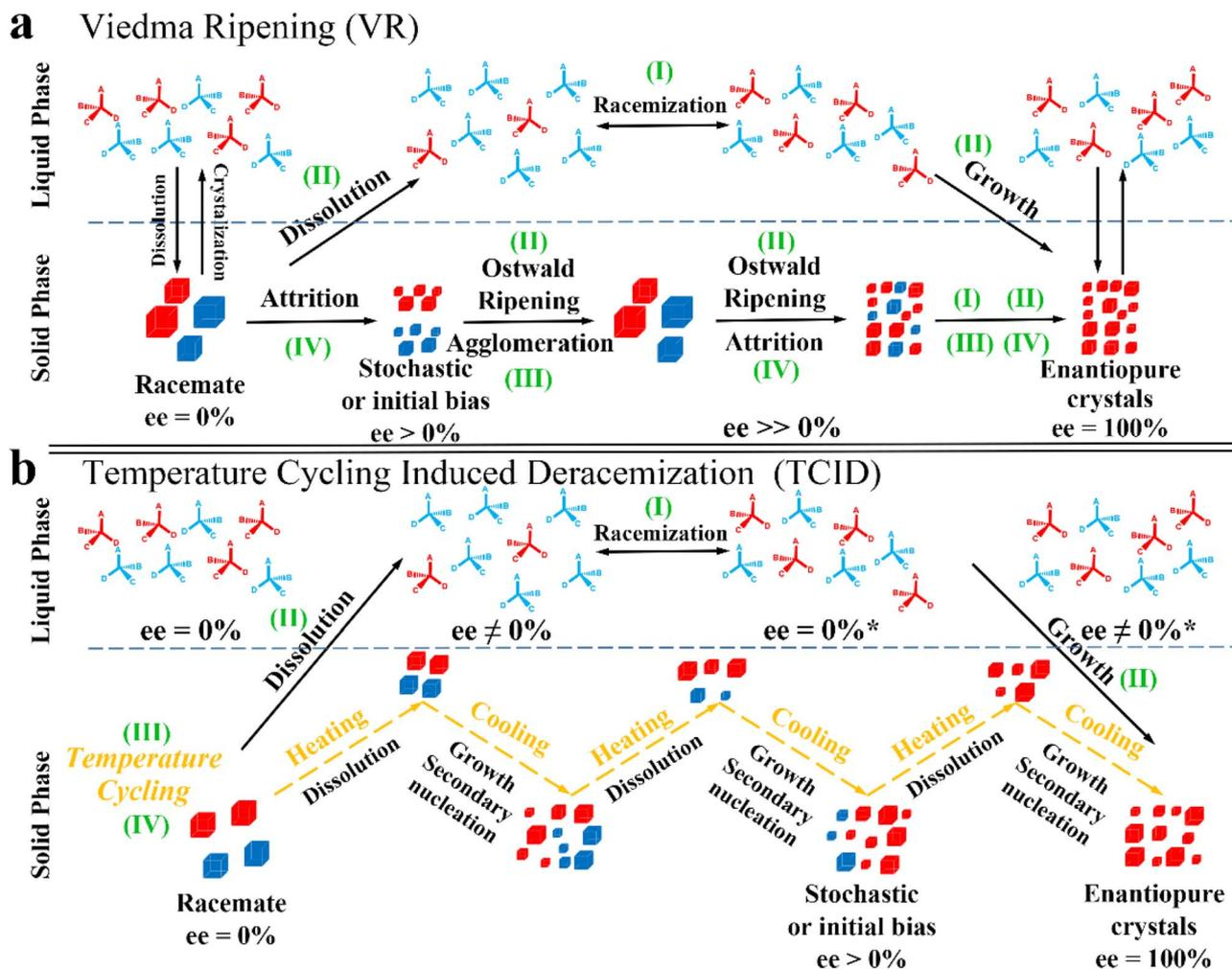
Fig. 15 Schematic representation (a) VR and (b) TCID mechanisms of a Con.<sup>259</sup> (I–III) Represent racemization, Ostwald ripening and agglomeration/cluster incorporation, respectively. (IV) Represents attrition (for VR) or size/solubility differences resulting from temperature fluctuations (for TCID). Red and blue molecules represent D- and L-enantiomer, respectively.
