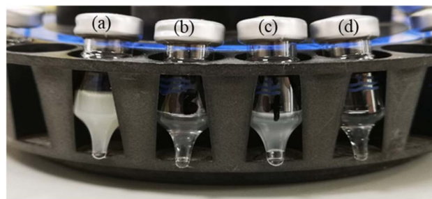
Fig. 6 The physical appearance of the final extractor of nitrofurans determination, (a) QC (without Hydrophobic CMCs), (b) CMC-C18, (c) CMC-C4, (d) CMC-C1.
