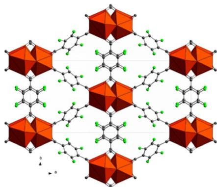
Fig. 9 Crystal structure of Ce-MIL140A, view along the *c* axis. Color code: cerium cluster orange, carbon grey, fluorine green.<sup>29</sup>
