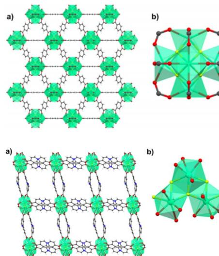
Fig. 4 On top: crystal structure of Ho-UiO-66 MOF. (a) Extended view along the *a* direction. (b) Holmium hexacluster containing  $\mu_3\text{-F}$  bridging groups. Reprinted with permission from ref. 44. Copyright 2021 American Chemical Society. On the bottom: crystal structure of Ho-4,4′-BPDC MOF. (a) Extended view along the *a* direction. (b) Holmium tricluster containing one  $\mu_3\text{-F}$  group. Reprinted with permission from ref. 44. Copyright 2021 American Chemical Society.
