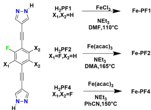
Scheme 3 Synthetic conditions for the preparation of the three fluorinated bis(pyrazolyl)-based MOFs.<sup>49</sup>
