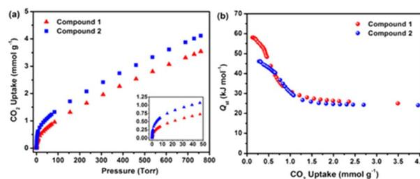
**Fig. 15** (a)  $\text{CO}_2$  data for 1 and 2 at 298 K. The inset shows the steep slope for 1 and 2 up to 50 Torr. (b)  $Q_{\text{st}}$  in 1 and 2 calculated from the 258, 273, and 298 K adsorption isotherms. Reprinted with permission from ref. 67. Copyright 2013 American Chemical Society.
