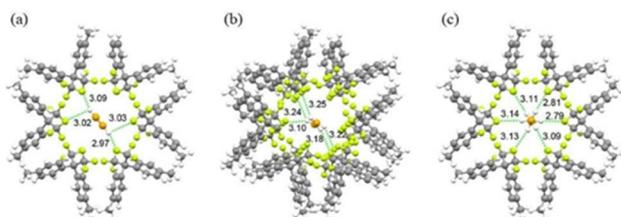
Fig. 16 DFT-D calculated (a)  $C_2H_2$ , (b)  $C_2H_4$ , and (c)  $C_2H_6$  adsorption locations in Zn-FBA. The unit for bond length is Å, carbon, fluorine, and hydrogen atoms in the framework represented by grey, green, and white, respectively, carbon and hydrogen atoms in adsorbate represented by orange and white, respectively, carbon and hydrogen atoms in adsorbate represented by orange and white, respectively. Reproduced from ref. 48 with permission from John Wiley & Sons, copyright 2022.
