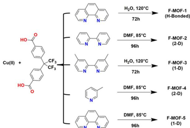
**Scheme 2** Reaction conditions for the syntheses of F-MOF-*x* from the work of Banerjee and co-workers.<sup>47</sup>
