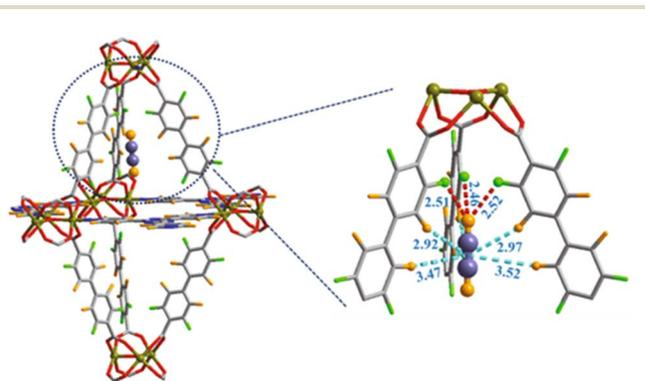
Fig. 17 Preferential C<sub>2</sub>H<sub>2</sub> adsorption site calculated from GCMC simulation for JXNU-12(F). Element key: Ni (dark yellow), C (gray), F (bright green), O (red) and H (bright orange). Reproduced from ref. 62 with permission from Elsevier, copyright 2022.
